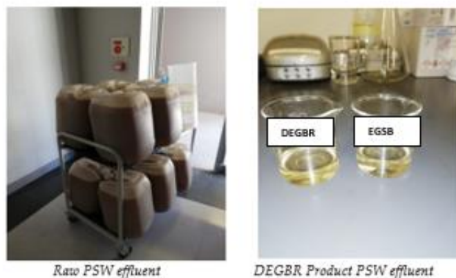
Figure 3-30: A comparison of Raw PSW effluent and DEGBR product sample
