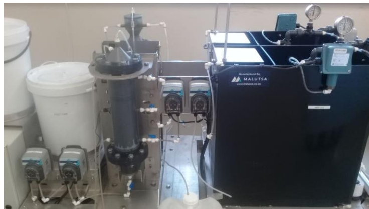
Figure 3-13: Photograph of the modified down-flow expanded granular bed reactor (DEGBR) (source: D.N. Dlamini)
