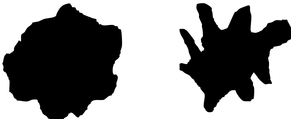
Figure 3.12: Assumed particle of A) GV40 with a smaller surface area but dense B) V40 with a larger surface area and less dense.
