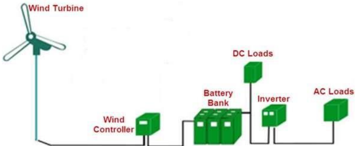
Figure 2.17: Battery Energy Storage System (Luo et al., 2015)
