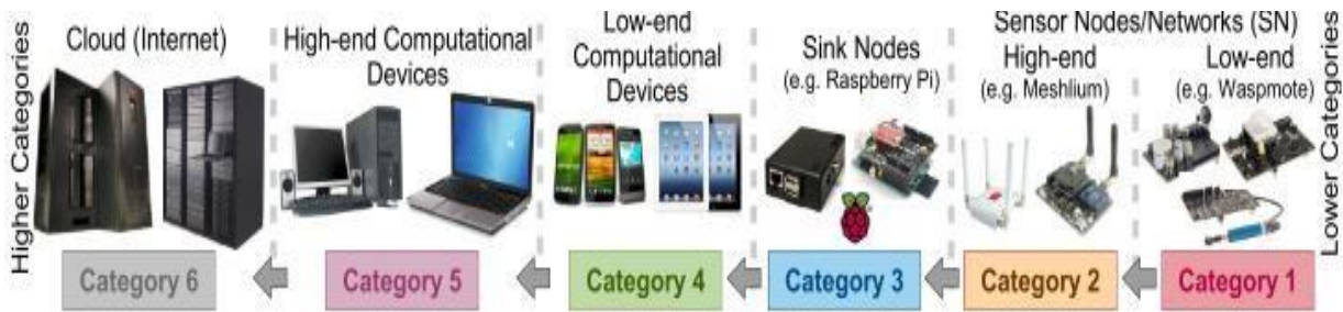
Figure 2.21: Classification of IoT devices centered on computational abilities, cost, and memory adapted from (Perera et al., 2014)
