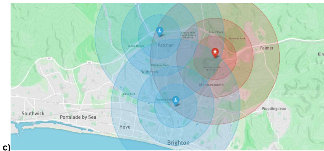
FIGURE 2.8 A) FIXED LOCATION SPECTRUM MONITORING SYSTEM B) LS TELCOM MONITORING TOWER C) LS THEORETICAL COVERAGE OF SPECTRUM MONITORING TOWERS
