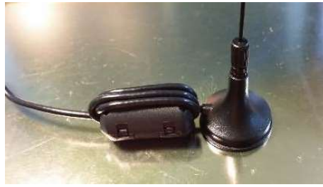
FIGURE 3.8 FERRITE COAX CHOKE ADDED TO THE ANTENNA CABLE
