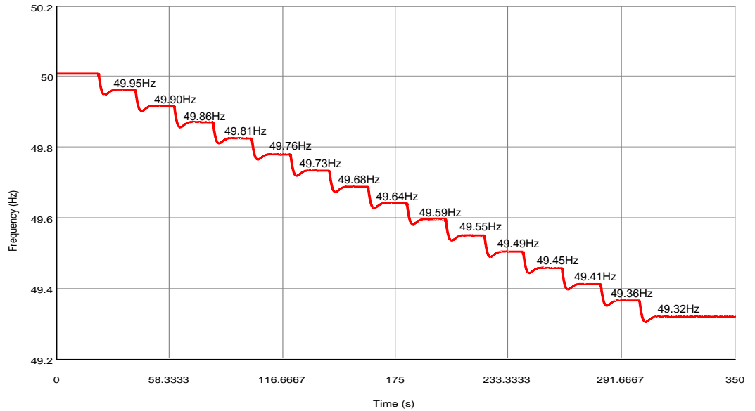
Figure 7.7: System frequency during speed governing system response
