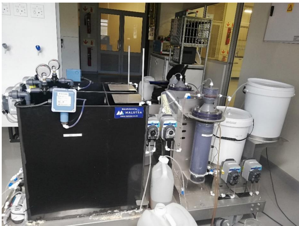
Figure 3. 1: Poultry slaughterhouse wastewater (PSW) miniaturized lab-scale plant setup.
