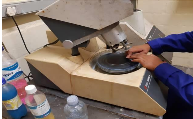
Figure 3. 8: Polisher machine used in preparation of microscope samples
