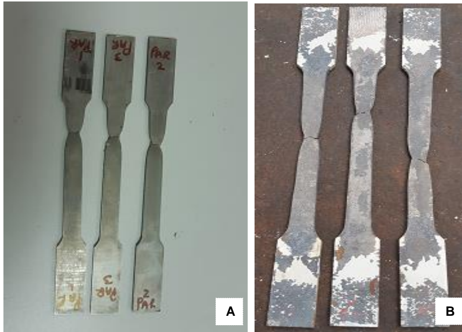
Figure 4.5: Fractured tensile samples, (A) Parent, (B) 60 Minutes
