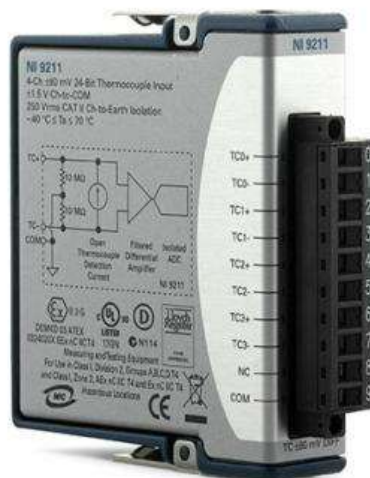
Figure A.2:2. NI 9211C Series Temperature Input Module
