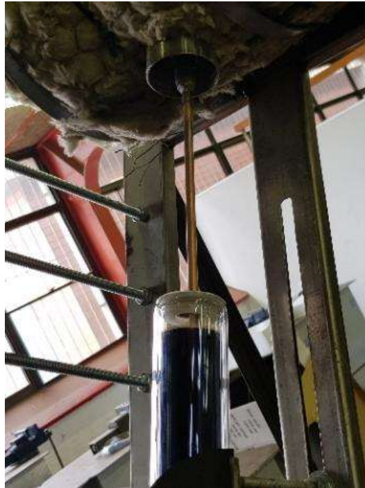
Figure 4.5: Heat pipe screwed into the water tank
