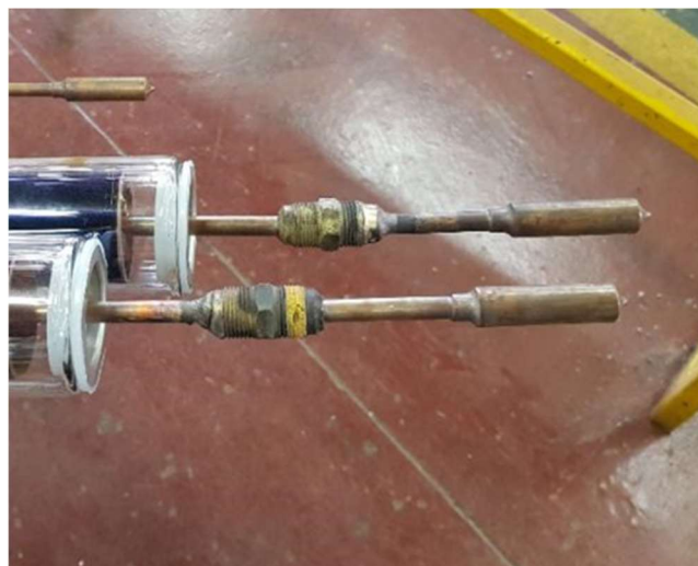
Figure 4.6: BSP male thread welded on the heat pipe
