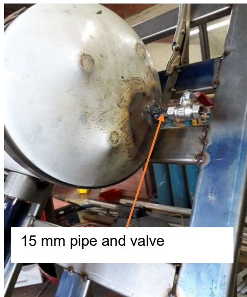
Figure 4.4: 15 mm pipe and valve
