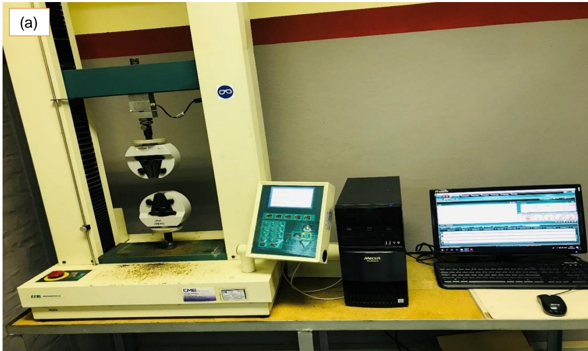
Figure 3.7.1: (a) Hounsfield 50 K testing machine (Used for Tensile test).
