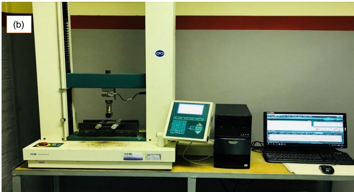
Figure 3.7.1: (b) Hounsfield 50 K testing machine (Used for the Bending test).
