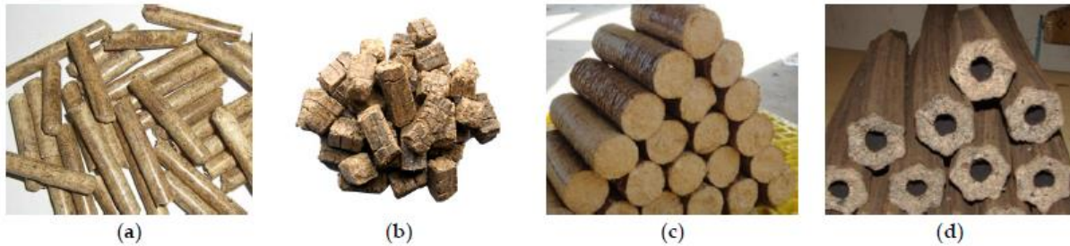
Figure 2.5: Common biomass shapes and sizes of briquettes; (a) Pellet (b) Briquette (c) Solid rod (d) Hollow rod (Xu et al., 2015).
