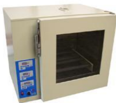
Photograph 3-10: Shaking incubator, ISKO 80, FMH instruments, Cape Town South Africa
