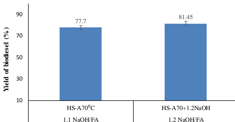
Figure 6. 1. Yield of maggot oil-derived biodiesel as a function of NaOH/CFA ratio in catalyst synthesis (Trans. conditions: 60 °C; 15:1 MeOH/oil ratio; 600 rpm; 1.5 % catalyst wt. and 1.5 h) (NaOH/FA= NaOH/CFA)
