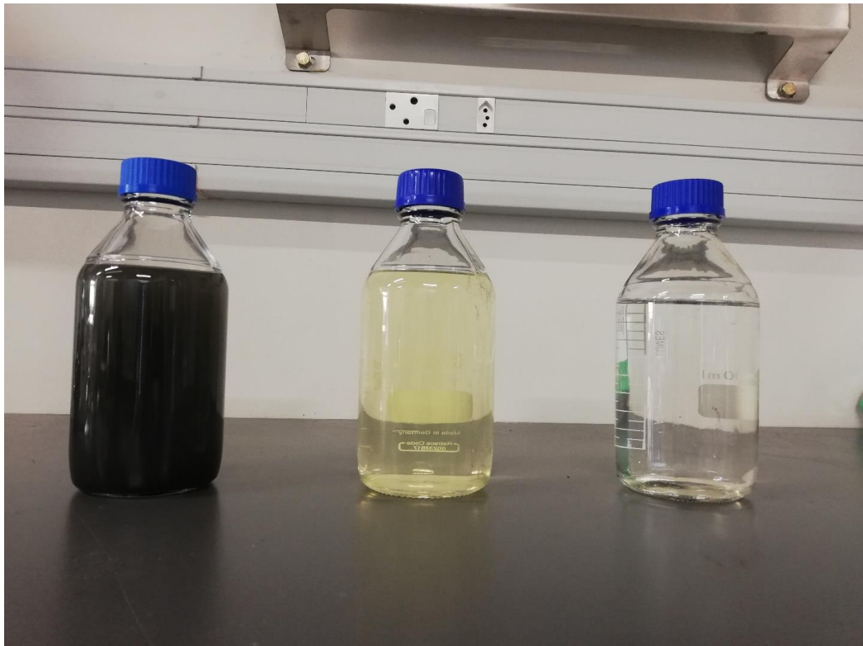
Photograph 4- 3: Initial, Coagulation, and Electrochemical Oxidation
