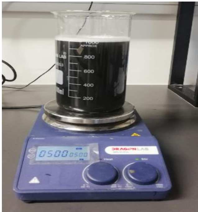
Photograph 3- 1: Initial Carwash Wastewater in Coagulation process
