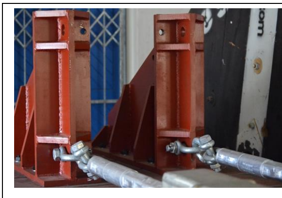
Tensioned the conductor, Figure 4. 3: Rigid Support Sityoshwana, 2019
