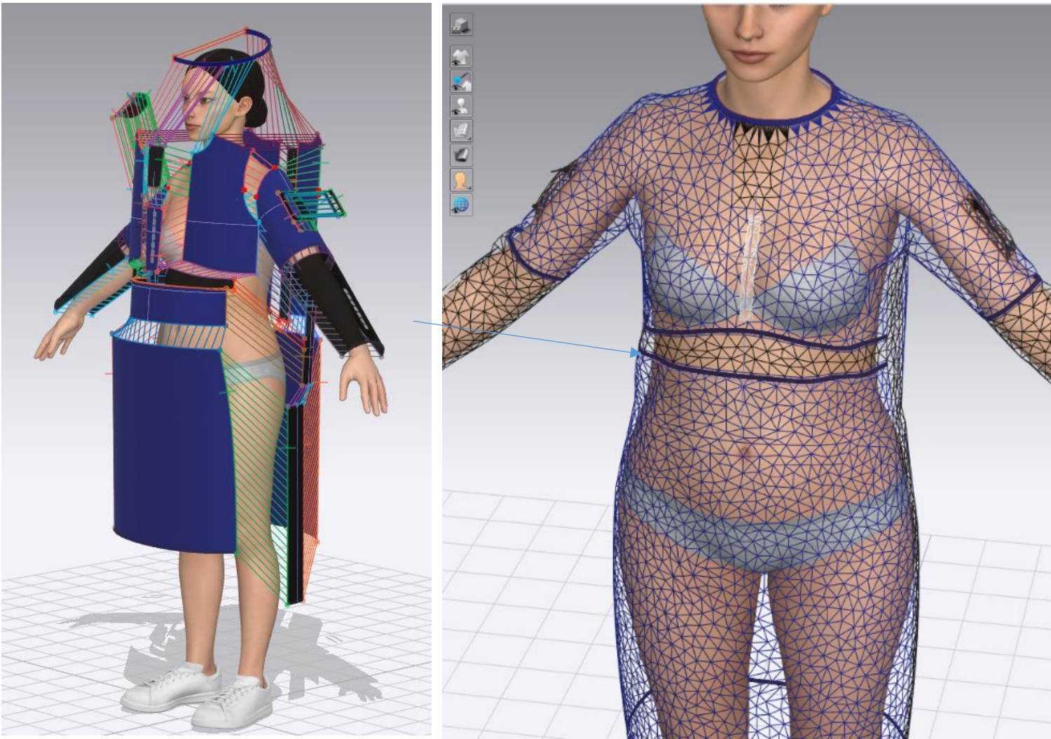
Figure 5. 12 Pattern arrangement, stitching (left) and ease allowance (right) (Author, 2019)
