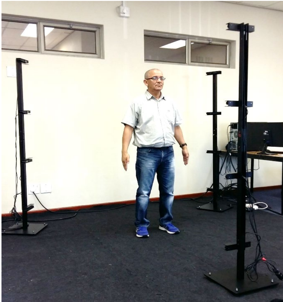
Figure 2. 2 Human Solutions Anthroscan 3D scanner (Author, 2018)
