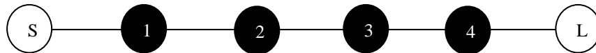
Figure 6.3: Normalised coupling matrix M and schematic topology of the fourth order filter without transmission zeros
