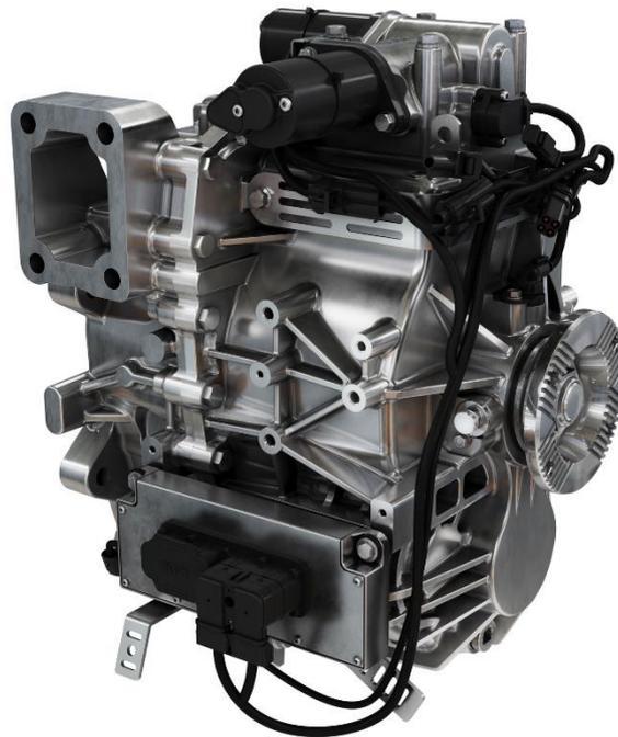
Figure 50. Eaton 4-speed EV transmission (Eaton, 2021).
