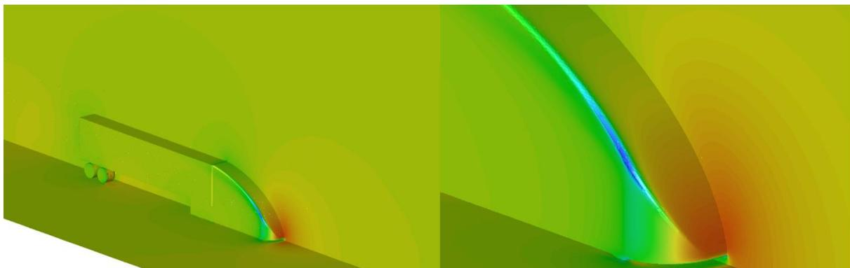
Figure 70. Flow pressure coefficient over Concept Two (left), and a magnified view of the frontal area (right).
