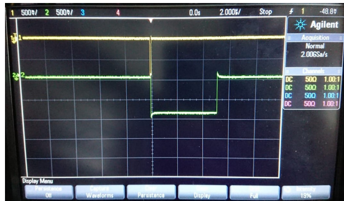
Figure 5.5: QDC busy time output signal (green)
