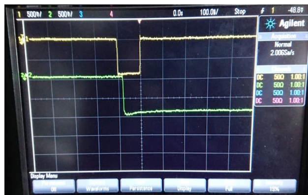
Figure 5.6: Trigger (yellow) with QDC busy time (green)
