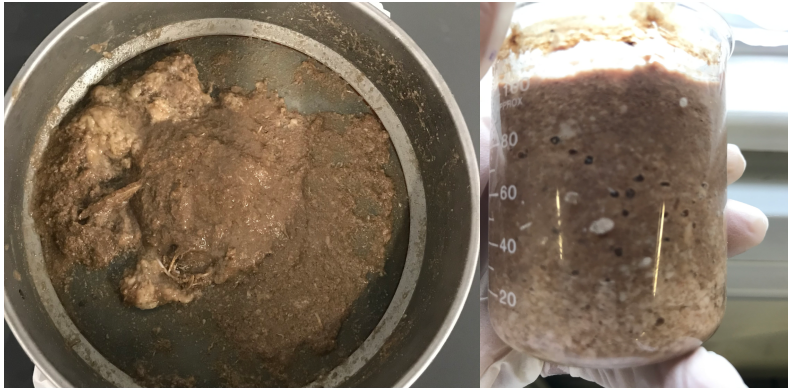
Figure 3:3: Suspended solids collected after sieving the pre-treated water
