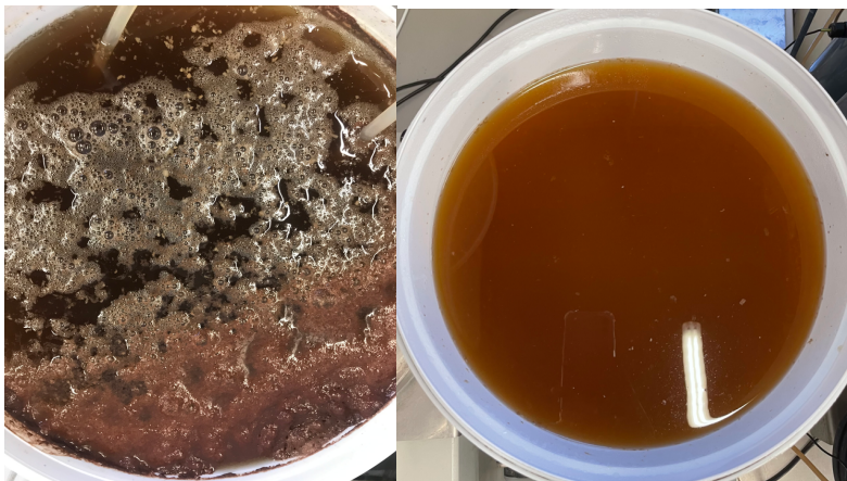
Figure 3:2: Pre-treatment stage of raw wastewater before and after sieving
