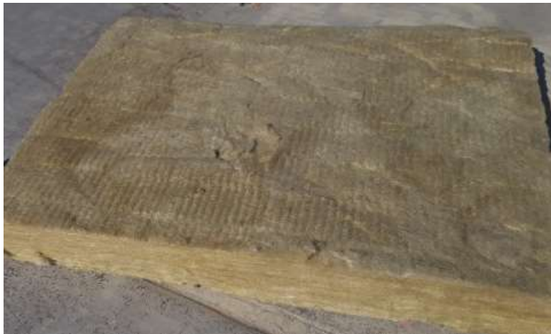
Figure 3.57: A 50mm thick glass wool insulation material
