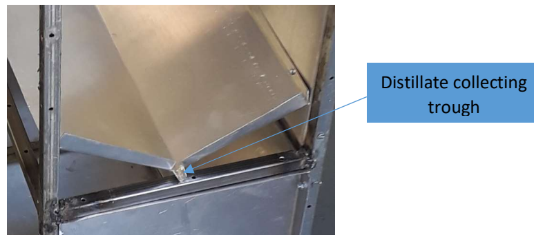
Figure 3.36: Distillate collecting trough
