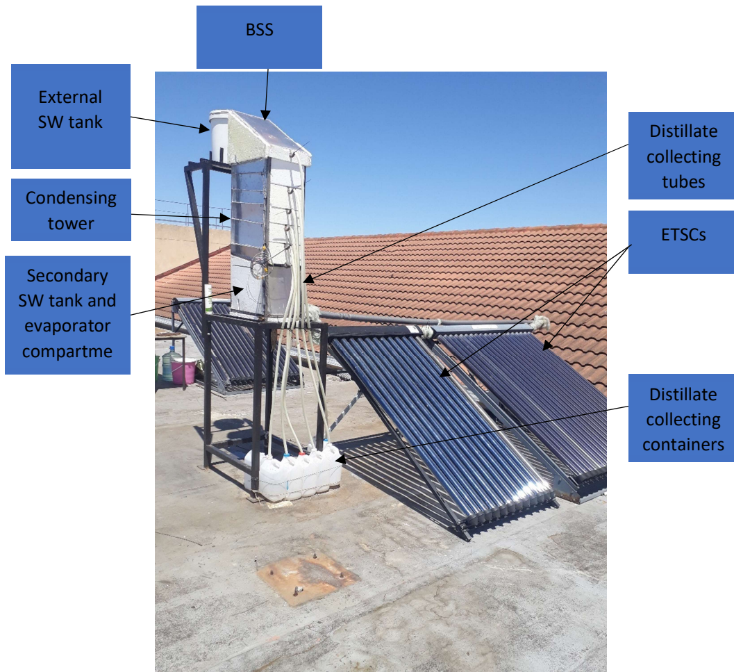
Figure 4.1: Vapour-based MSS-SS
