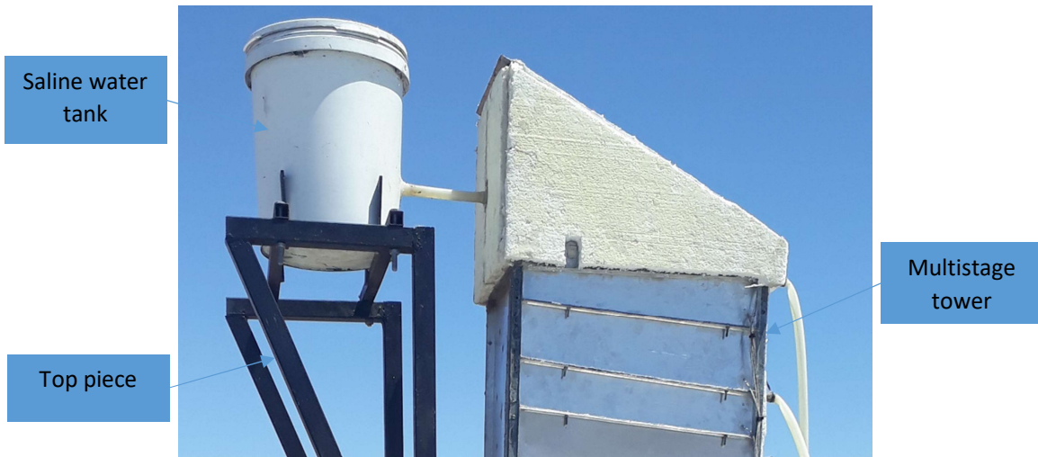
Figure 3.8: External saline water tank connection
