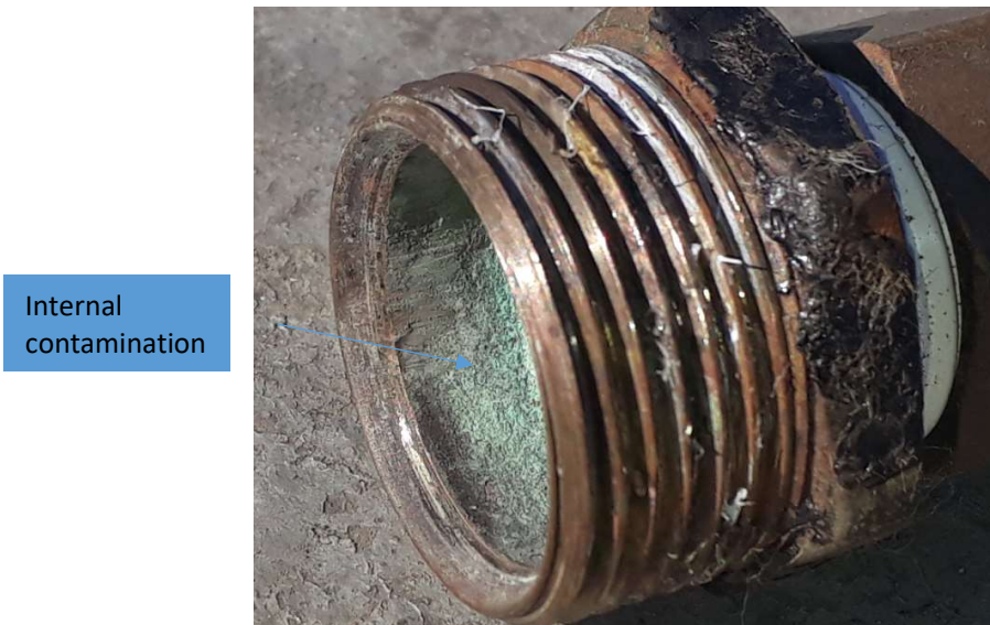
Figure 5.52: ETSC series connector contamination
