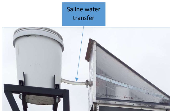
Figure 3.9: External tank saline water transfer tube
