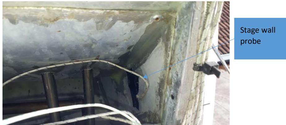
Figure 4.12: Surface probes attached onto stage 2 wall
