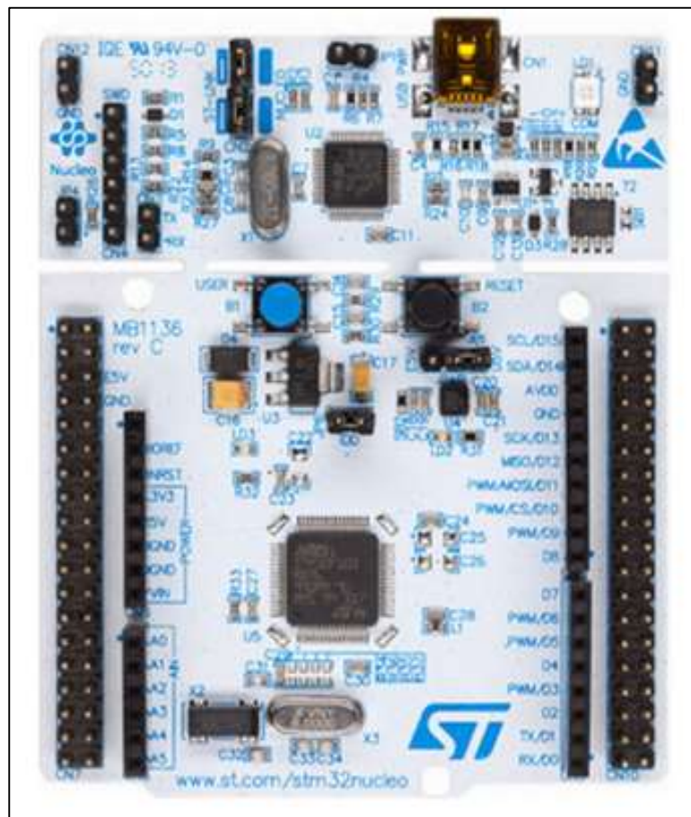
Figure 30: Nucleo-64 Development board.
