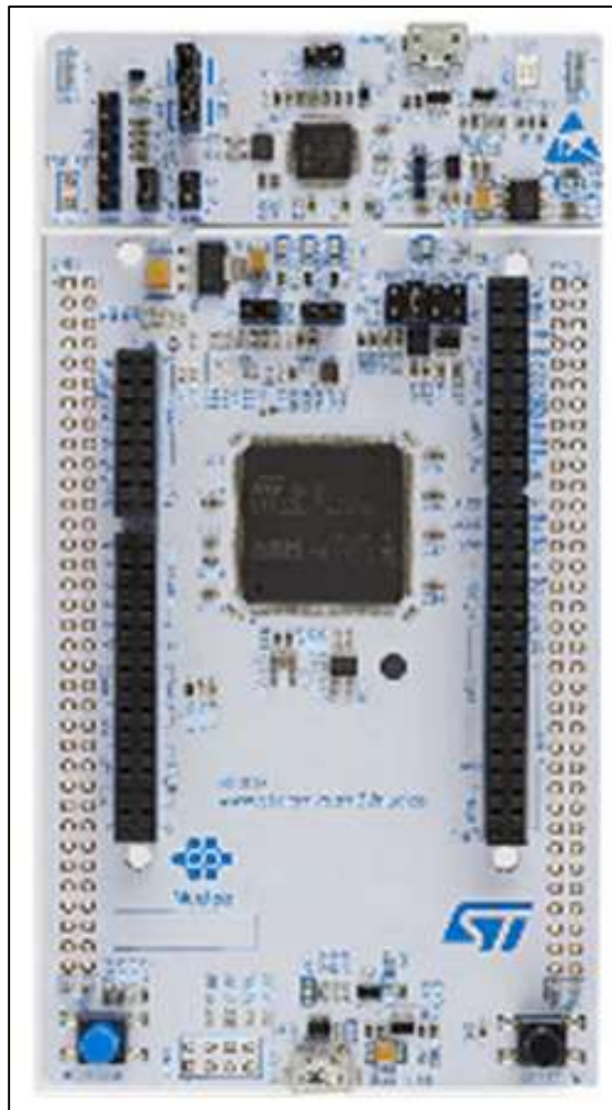
Figure 31: Nucleo-144 Development board.
