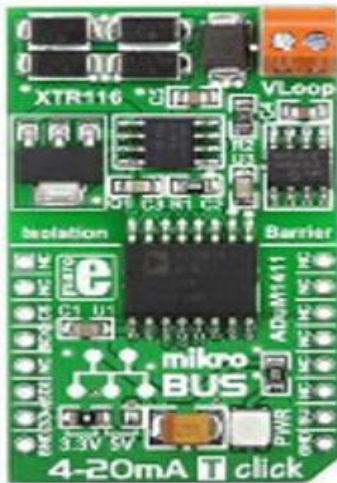
Figure 4.2: Module for measuring sensors 4-20mA with SPI interface.
