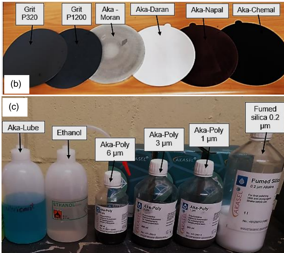
Figure 3.3.3: (a) Polishing machine; (b) polishing discs; (c) polishing agents.
