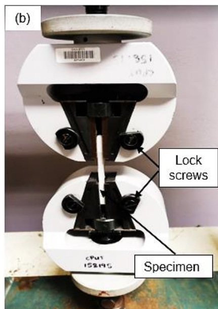
Figure 3.6.1(b): Tensile testing flat jaws.
