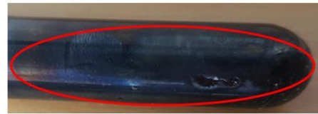
Puncture and burn marks on glassy carbon electrode (HV potential side)
