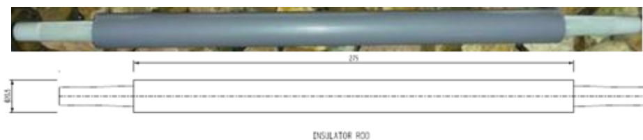
Figure 3-1: HTV-SR extruded onto glass fibre test samples (6x)
