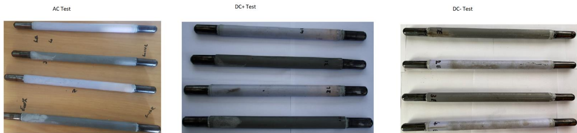
Figure 5-6: Overview of visual observations made (on RTV-SR and HTV-SR test samples) under AC, DC+, and DC- excitation voltages after the 6-day testing period
