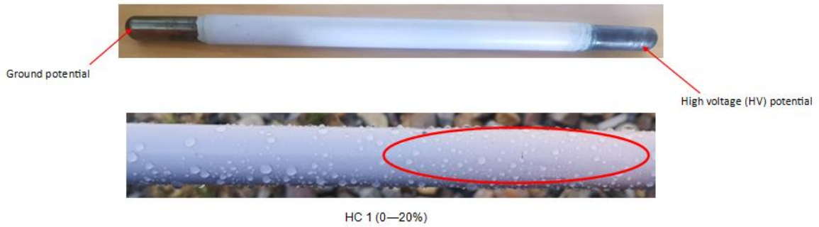
Figure 5-26: Hydrophobicity of the RTV-SR sample 4
