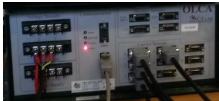
Figure 4-9: Front view of the OLCA used as a leakage current data logging device
