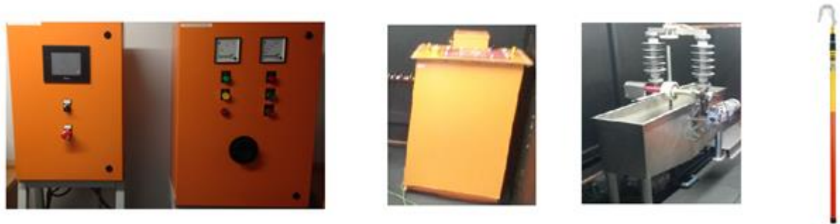
Figure 4-2: Overview of the test apparatus inside insulated shipping container: (a) control panels (b) 30 kV transformer and DC rectifier (c) RWDT and (d) HV earth stick
