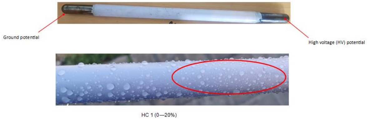
Figure 5-16: Hydrophobicity of the RTV-SR sample 2
