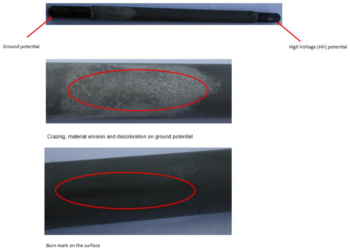
Figure 5-54: Discoloration, material erosion, crazing and dark pollution/contamination build-up on the HTV-SR test sample
