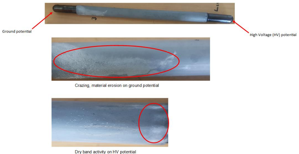
Figure 5-20: Traces of dry band activities, crazing and material erosion on HTV-SR test sample
