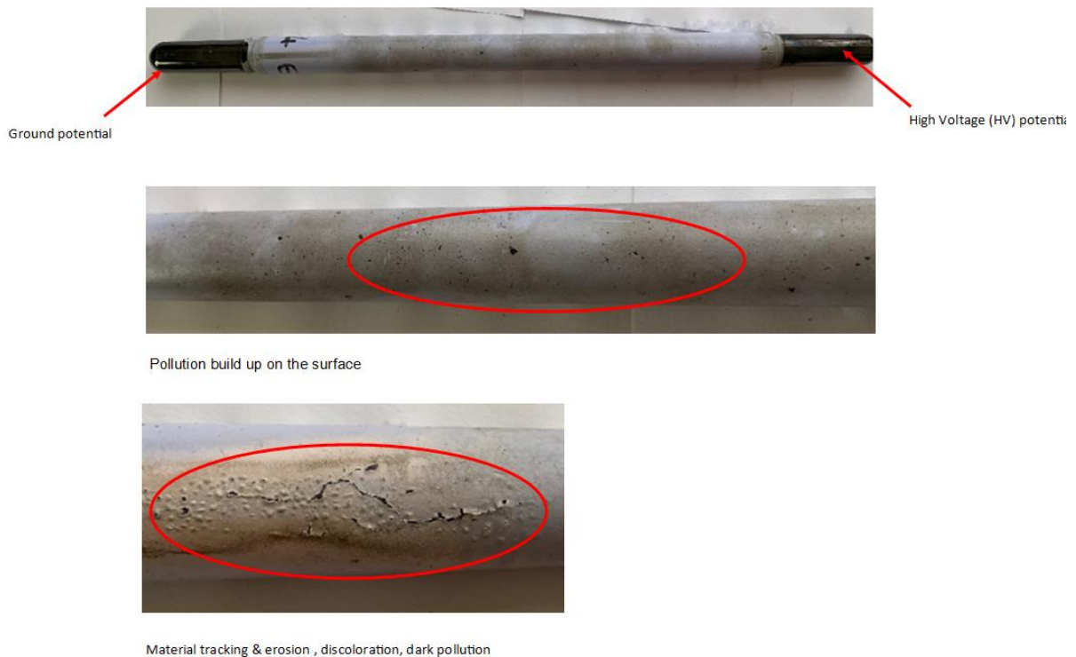
Figure 5-47: Material erosion, pollution, and discolouration on RTV-SR test sample
