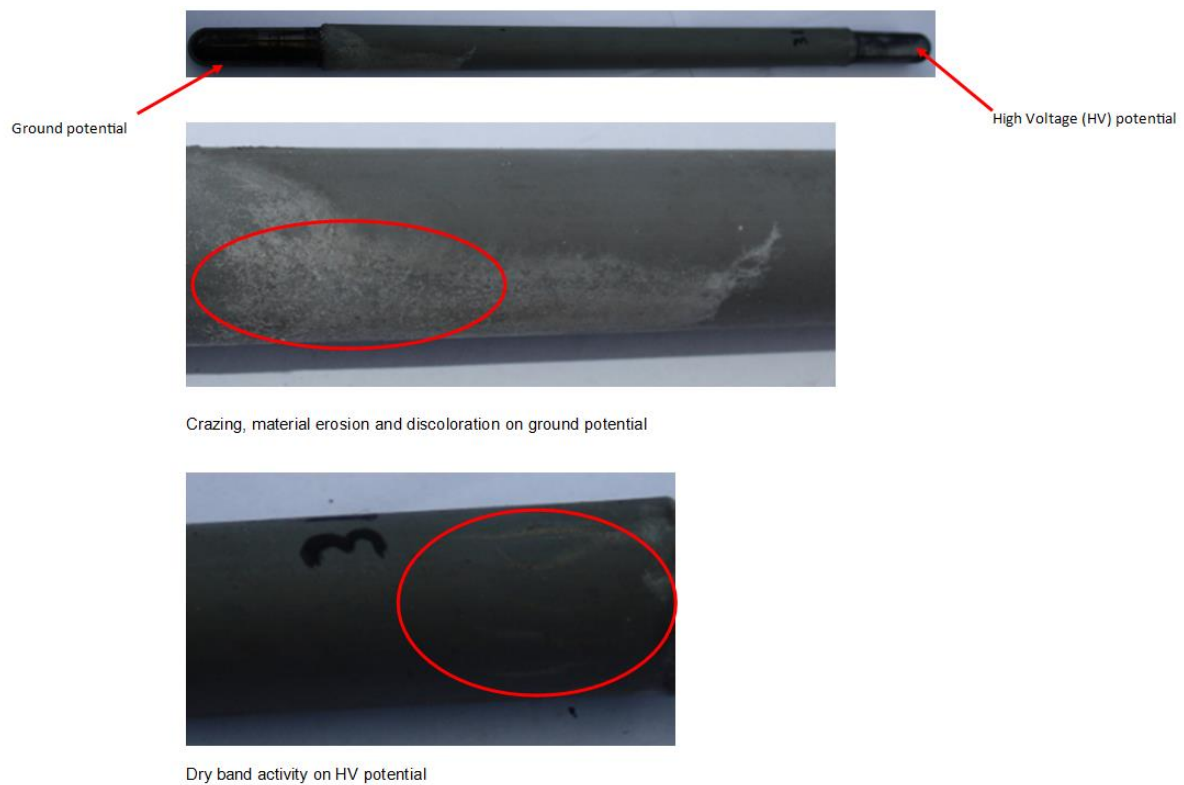
Figure 5-64: Dry band activity on HTV-SR test sample
