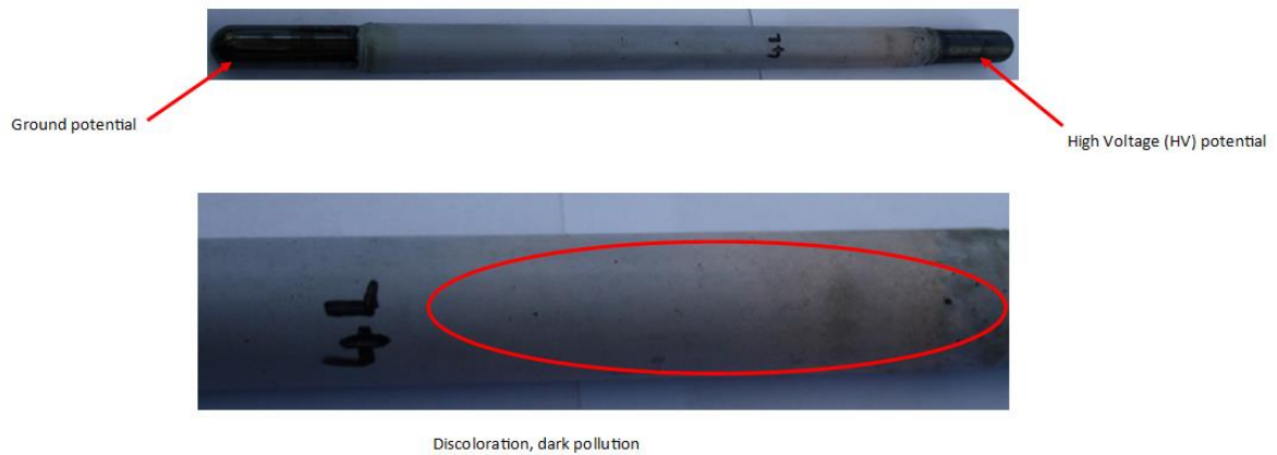
Figure 5-69: Discolouration, burn marks and pollution observed on an RTV-SR test sample
