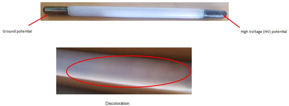
Figure 5-25: Tracking and erosion, discoloration, and pollution on RTV-SR test sample
