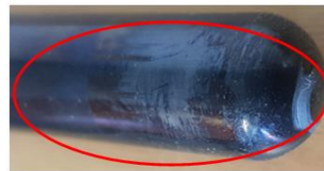
Crack and burn marks on glassy carbon electrode (HV potential side)
