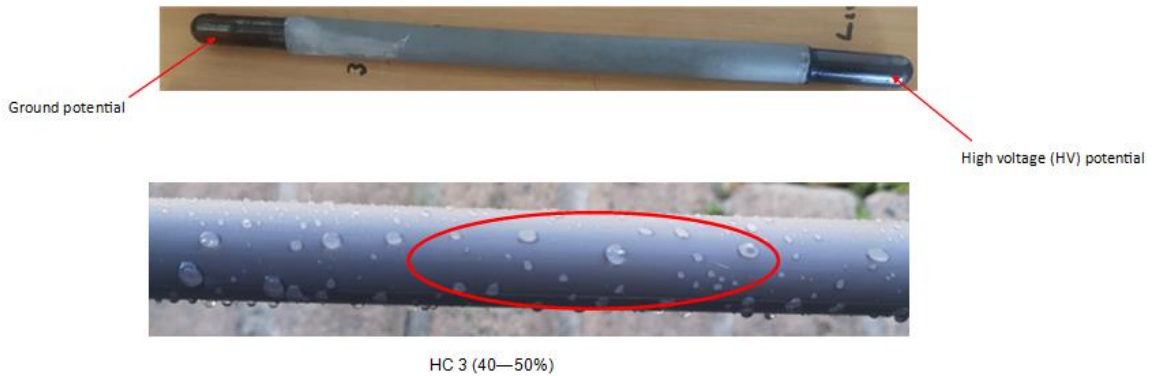
Figure 5-21: Hydrophobicity of the HTV-SR sample 3
