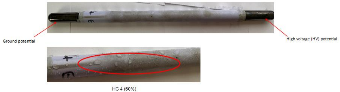
Figure 5-48: Hydrophilicity of the RTV-SR sample 8
