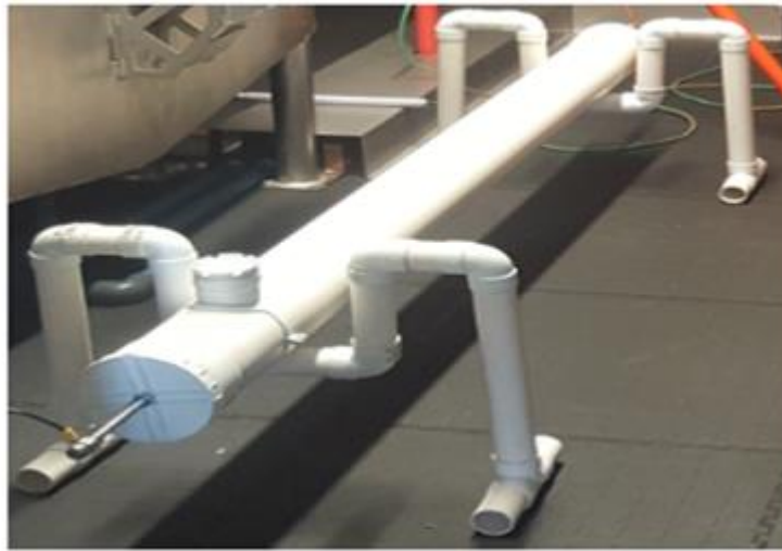
Figure 4-7: Fully constructed sodium chloride (NaCl) water resistor
