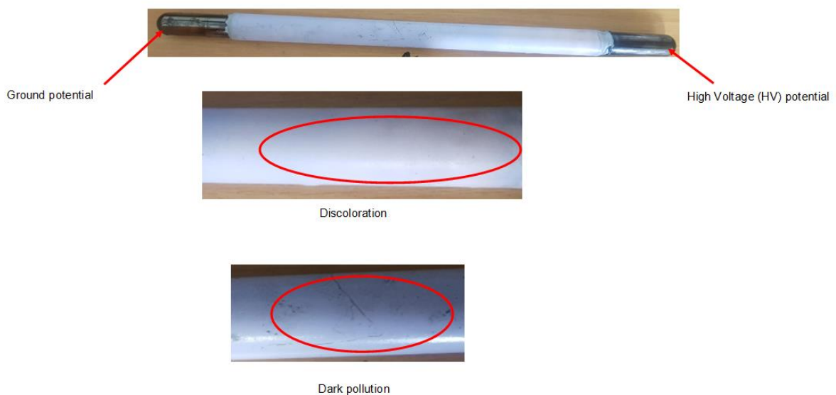
Figure 5-15: Dark pollution build-up and discolouration on RTV-SR test sample
