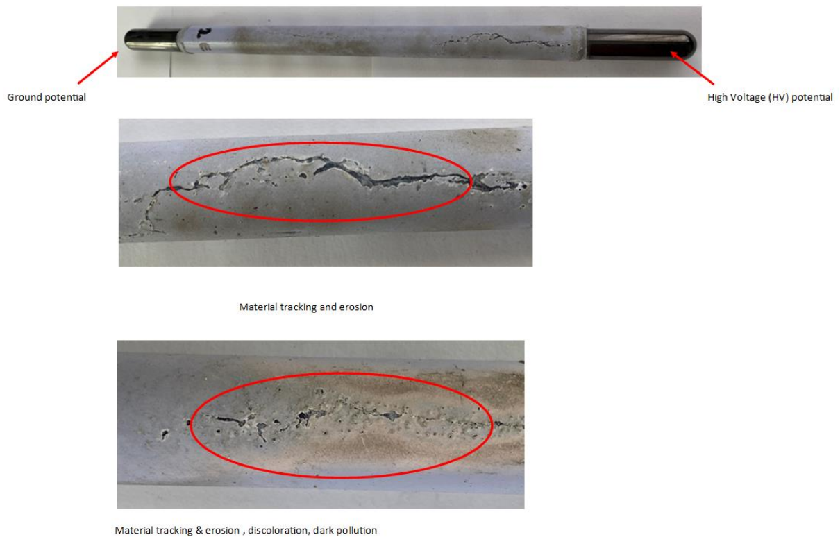
Figure 5-37: Black marks, burn marks on glassy carbon electrode, discoloration, and pollution on RTV-SR test sample
