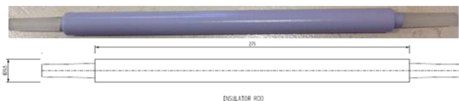
Figure 3-2: RTV-SR coated borosilicate glass test samples (6x)
