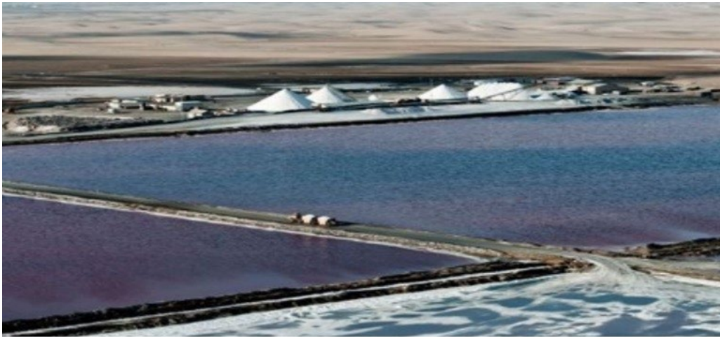
Figure 4.7: Solar evaporation in the production of salt at the WBSH mine (WBSH, 2019)
