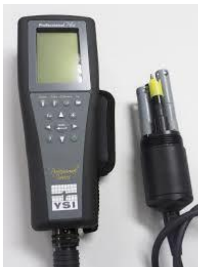
Figure 3.2.2. YSI Professional Plus multiparameter water quality meter (taken from Van Walt, 2019)
