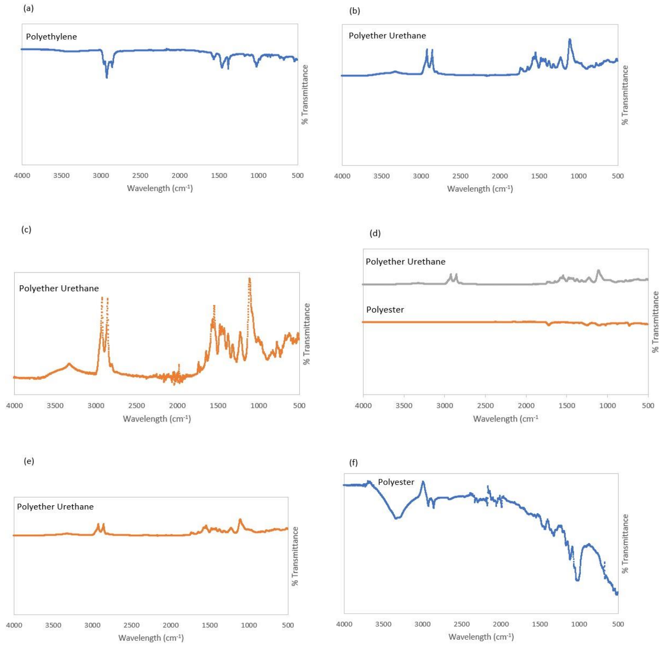
Figure 4.15: FTIR spectra of microplastics found in (a) Influent; (b) Effluent; (c) Point of discharge; (d) Upstream; (e) Downstream and (f) Sludge at the various sites in the WWTP and Veldwachters River
