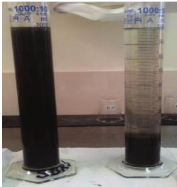
Figure 3.1: Photograph of the sludge volume index (SVI) test being conducted in measuring cylinders before and after settling of the activated sludge.
