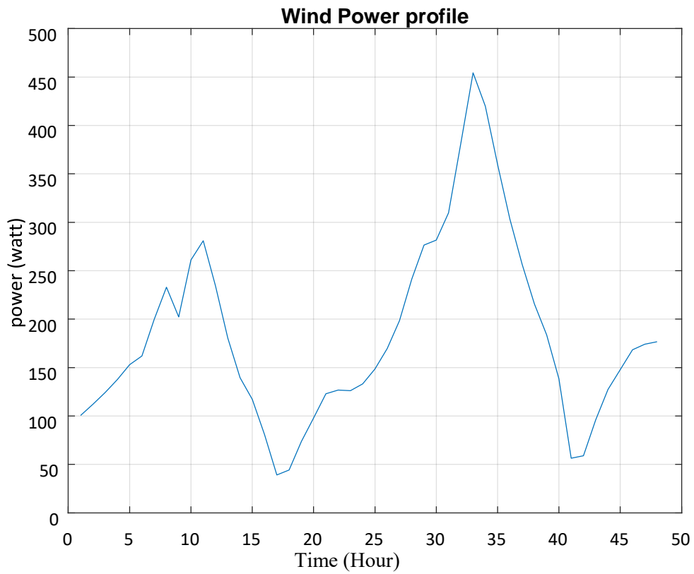
Figure 5.7: Hourly power output of the wind turbine
