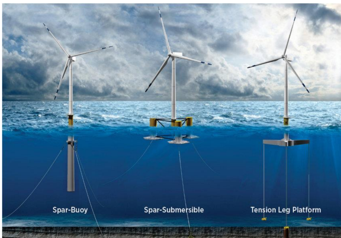
Figure 2.10: Three different floating options for offshore turbines (From Wisatesajja et al., 2019)
