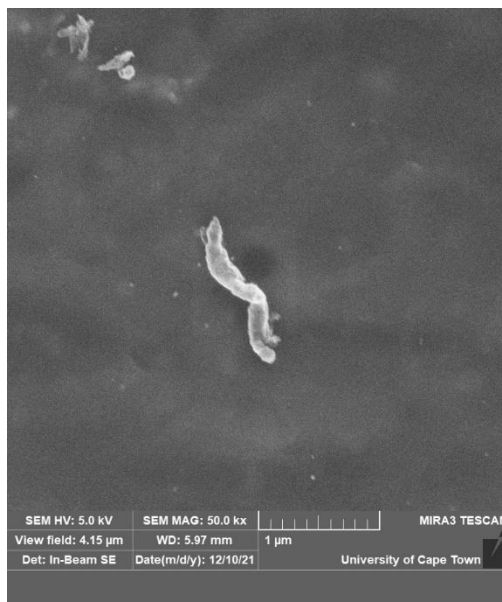
Figure H-38: SEM image of the top view of NF 10 bar, 44µg/l with a 50K magnification (Left) and a 10K magnification (right) after 100 hours.
