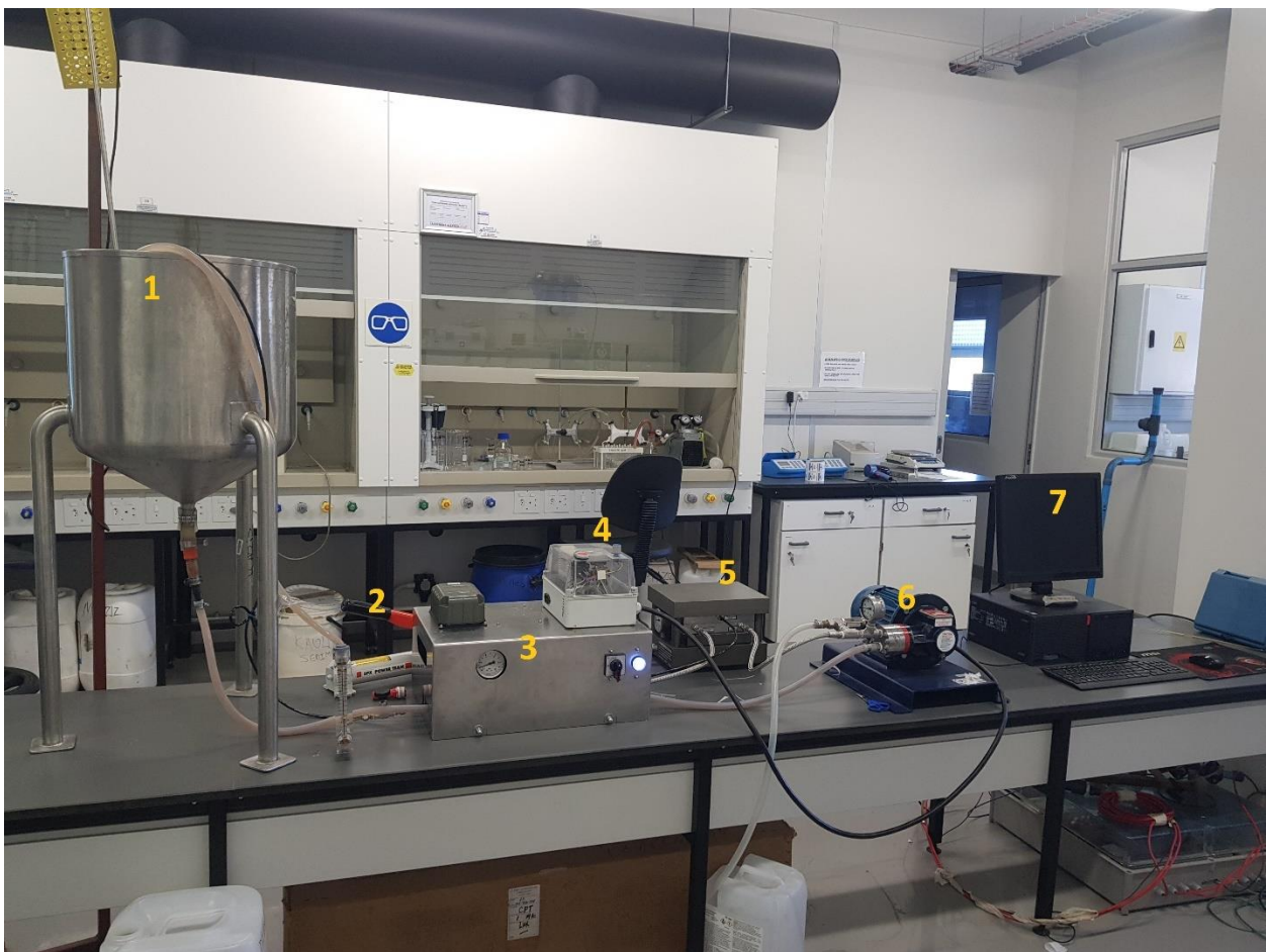
Figure 3-1: Bench-scale RO unit in Environmental Engineering Research Water Laboratory 1.18 (August 2021)
