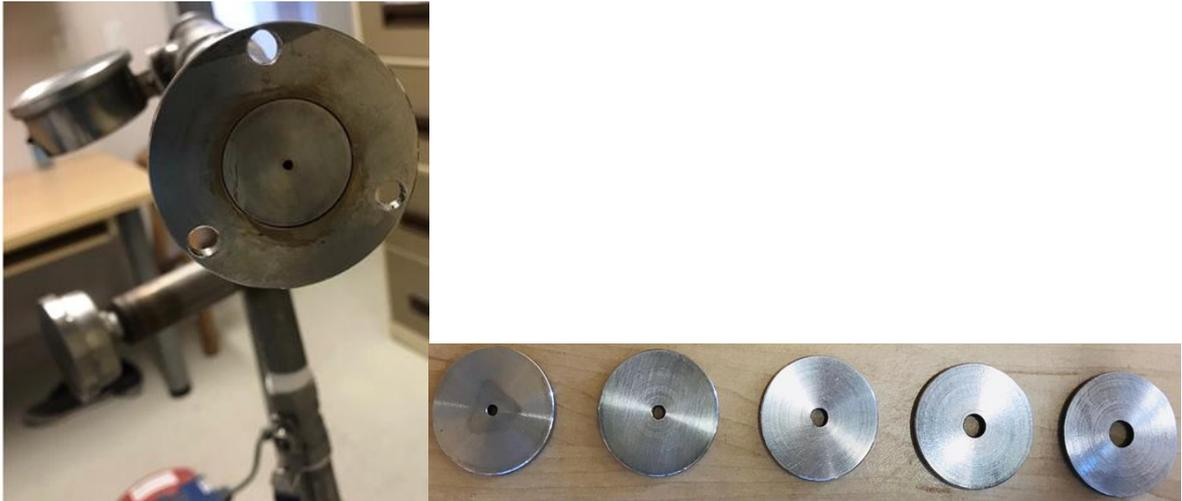
**Figure 3.5 Actual photograph of orifices cavitating device**
