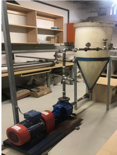
Figure 3.3 Actual photograph of hydrodynamic cavitation pilot plant
