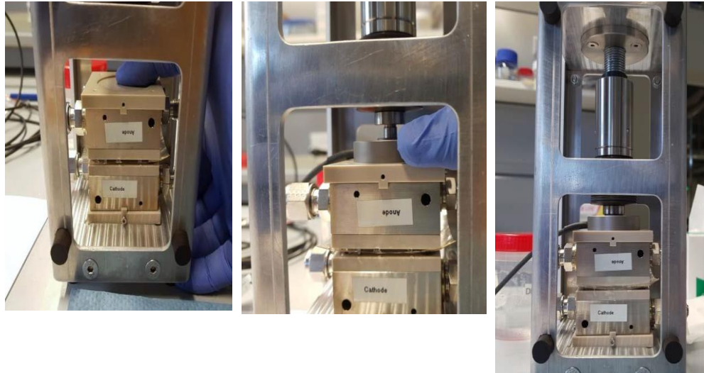
Figure 4.1.5: PEMWE cell insertion into compression frame.
