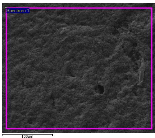
Figure 3.4.2: Anode catalyst layer surface images and their corresponding chemical compositions obtained from EDX analysis of (a) sample without pore former, (b) sample with Ammonium Carbonate and (c) sample with Ammonium Bicarbonate.
