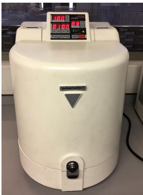
Figure 3.3.3: Roller mill machine used for anode electrode catalyst ink fabrication.
