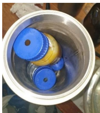
Figure 37: Sample bottles in the extractor basket
