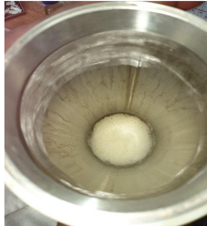
Figure 40: CO2 ice formation in extractor vessel due to fast depressurisation
