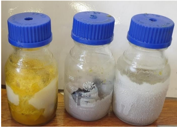
Figure 39: Frozen textile samples after fast depressurisation
