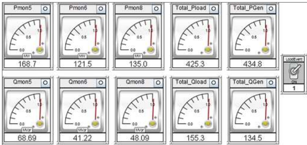
Figure 6 9: Metering of power after disturbance
