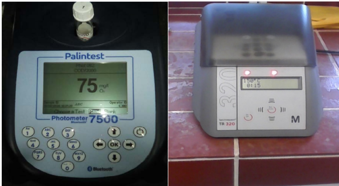
Figure 3.5 Palintest Photometer 7500 for measuring COD and a thermoreactor TR 320 for COD digestion process.
