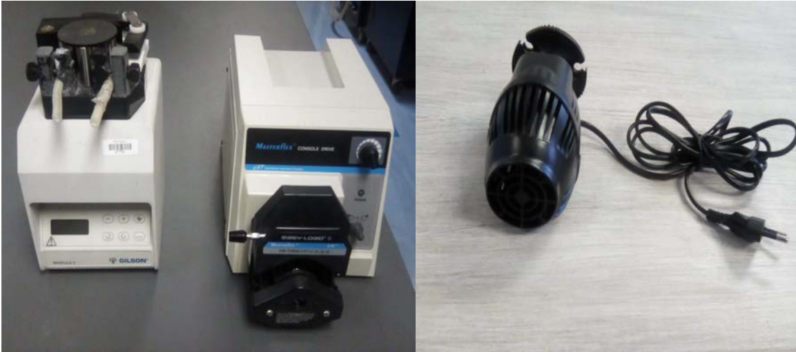
Figure 3.14 Peristaltic pumps (Gilson Minipuls 3 and cole Palmer 7520-40 console drive masterflex) and a submersible circulation wave pump (RS-108A).
