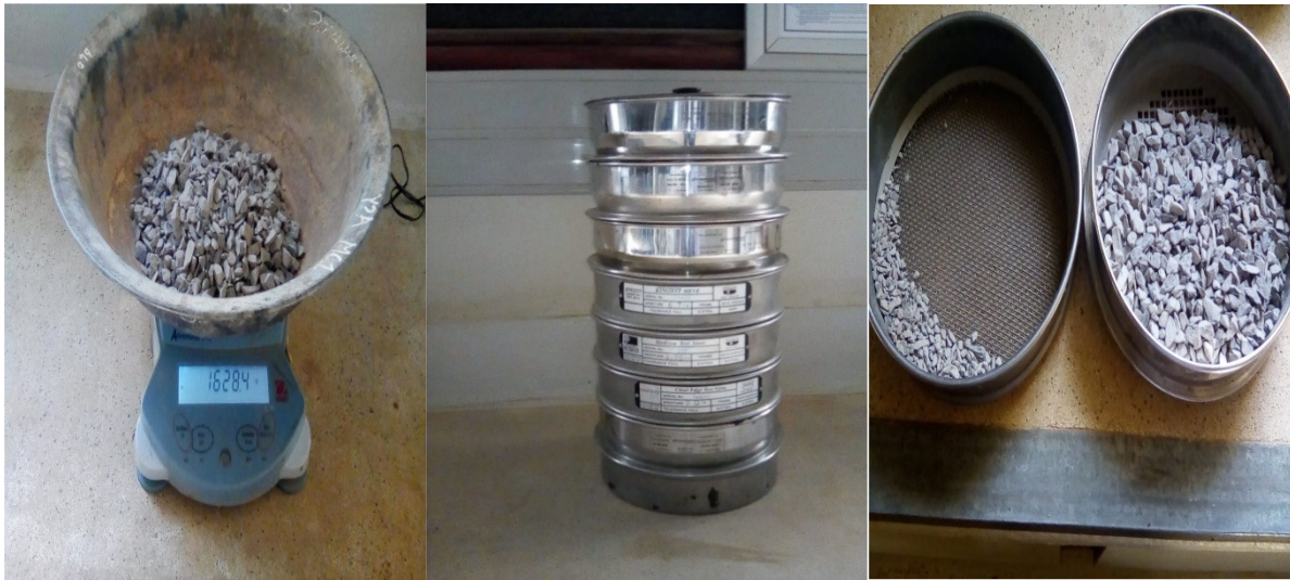
Figure 3.18 A sieve analysis to attain gravel filter gradation
