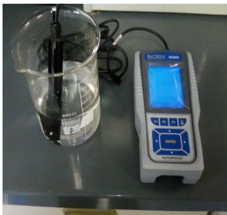
Figure 3.4 Cyberscan Dissolved Oxygen meter (Eutech DO 600) with a testing probe
