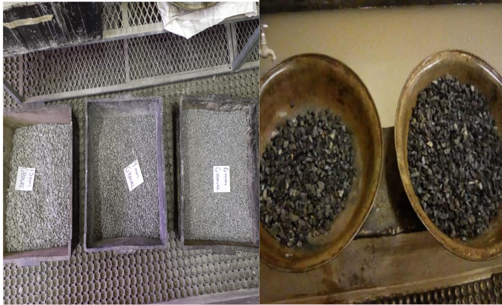
Figure 3.10 Granite gravel filter media size 13 mm, 9 mm, and 6 mm before and during cleaning off attached sand and clay particles.
