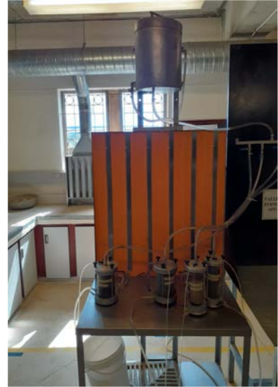
Figure 3.19 A schematic diagram and a laboratory setup of a constant head test.
