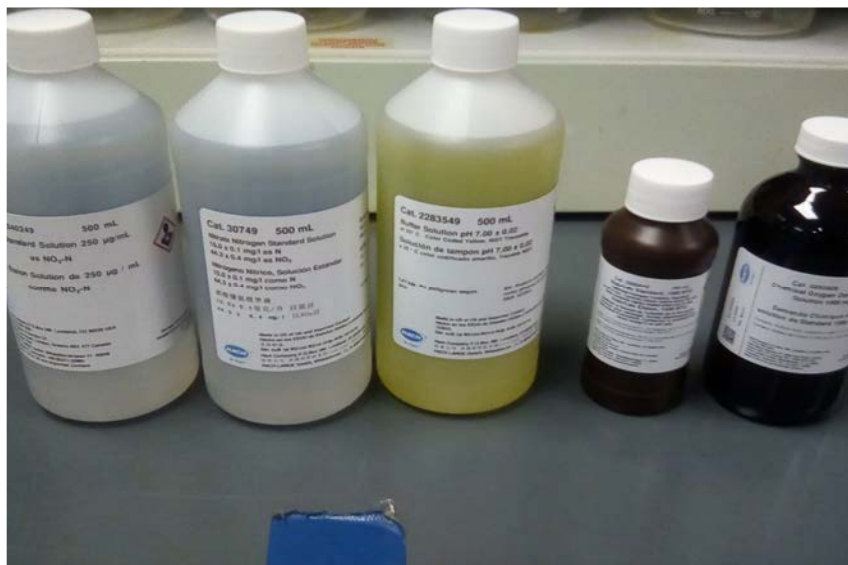
Figure 3.26 Standard solutions of known concentration for instrument verification
