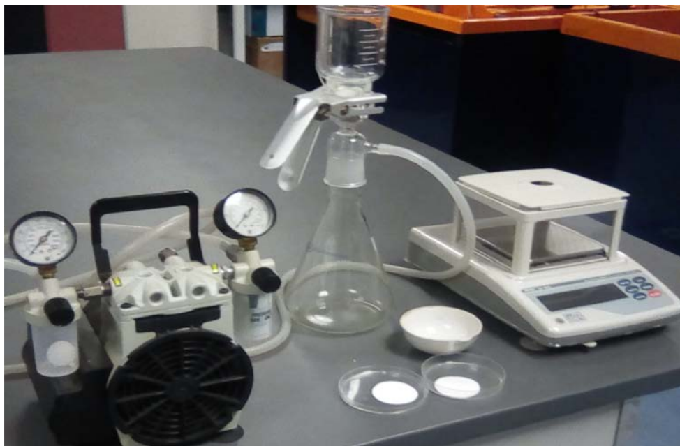
Figure 3.7 Standard duty piston pressure and vacuum pump (Model 2534), 1000 mL vacuum flask, filter paper and a laboratory analytical scale for TSS measurement.
