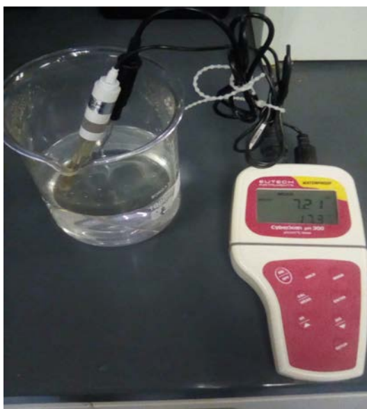
Figure 3.2 Eutech Cyberscan pH meter 300 fitted with a temperature test
