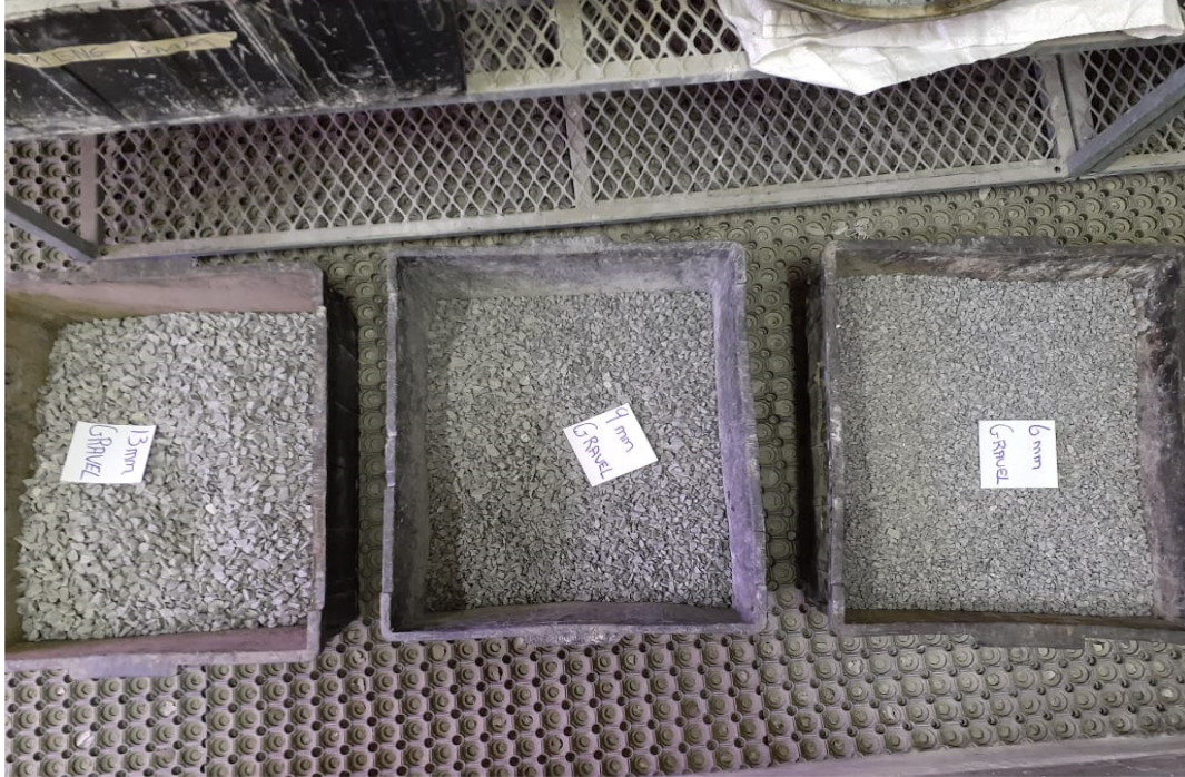
Figure 4.2 The 13 mm, 9 mm, and 6 mm filter media aggregates after sieving
