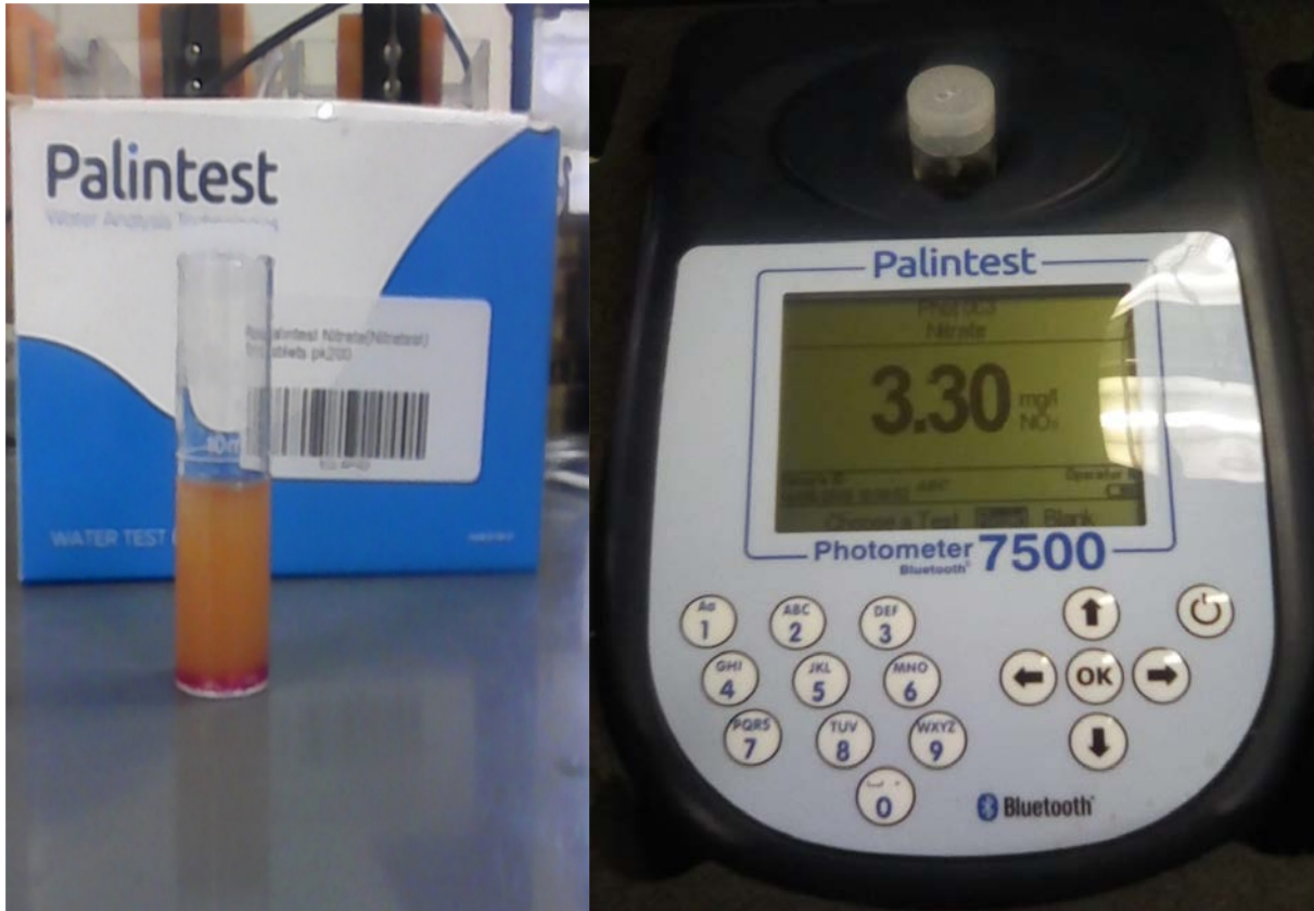
Figure 3.8 A Palintest tube test with reagents and Palintest Photometer 7500 for measuring nitrate and nitrite concentrations.
