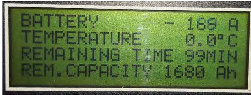
Figure 2.9.4: Remaining battery life indication on the control panel
