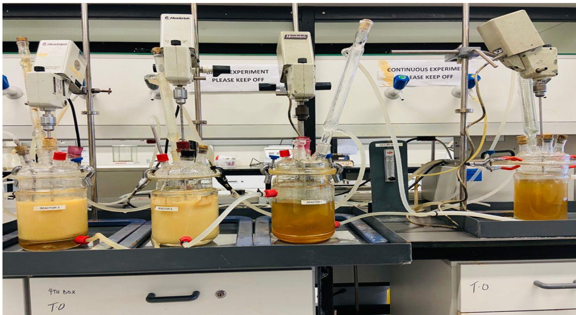
Figure 3.3: Stirred tank experimental set-up for ferrous ion bio-oxidation
