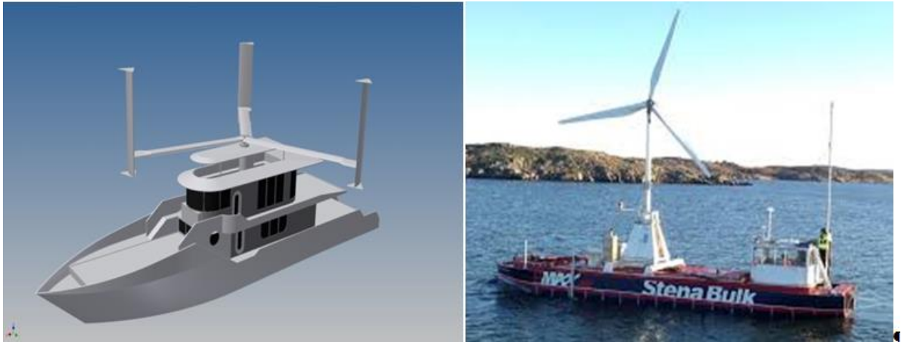
Figure 2.5: Example of typical wind turbines installed on the Ship (Carlso and Nilsson, 2015 )
