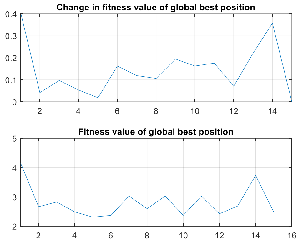
Fig. 6.21: 118-bus system convergence characteristics of the PSO algorithm after increasing termination condition tolerance of the change in the fitness value (top trace), showing successful convergence
