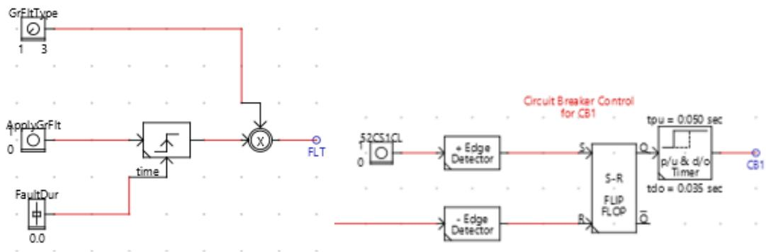
Figure 6. 10: Fault control logic.
