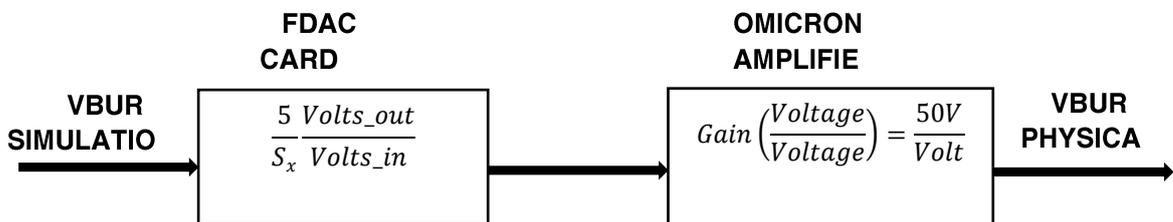
Figure 6. 5: The output scaling diagram for voltage signals
