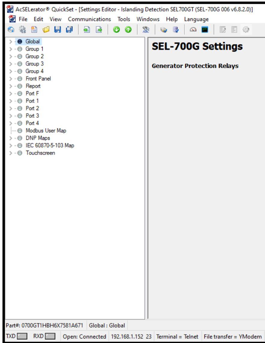
**Figure 6. 19: AcSErator QuickSet configuration window**
