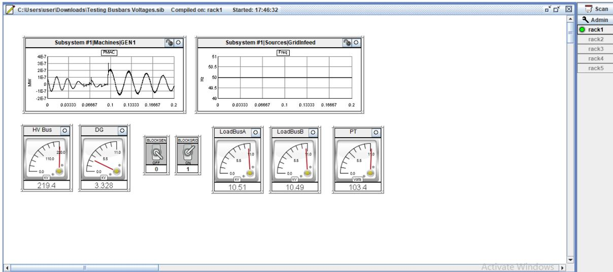
Figure 6. 13: DG circuit breaker open
