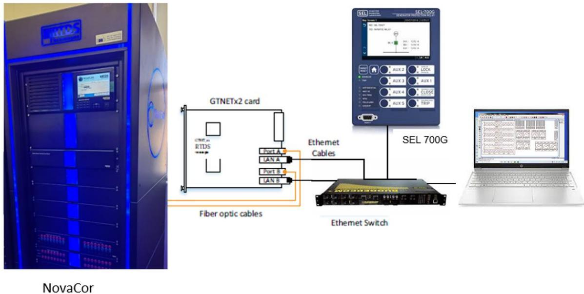
Figure 6.39: Connection of the GTNETx2-GSE-v7 to external device (IED)
