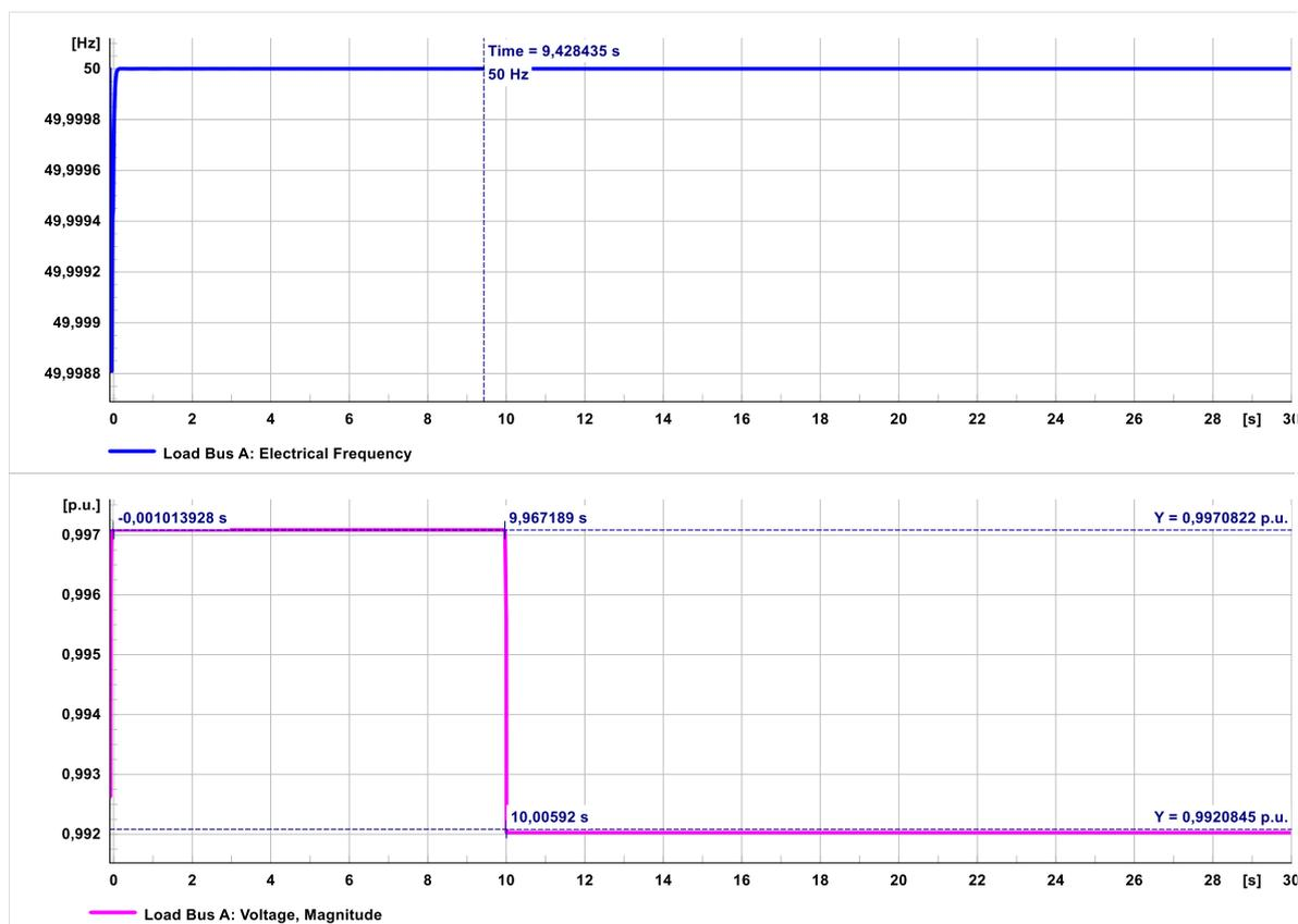
**Figure 4. 4: Network response when Grid Circuit breaker closed**
