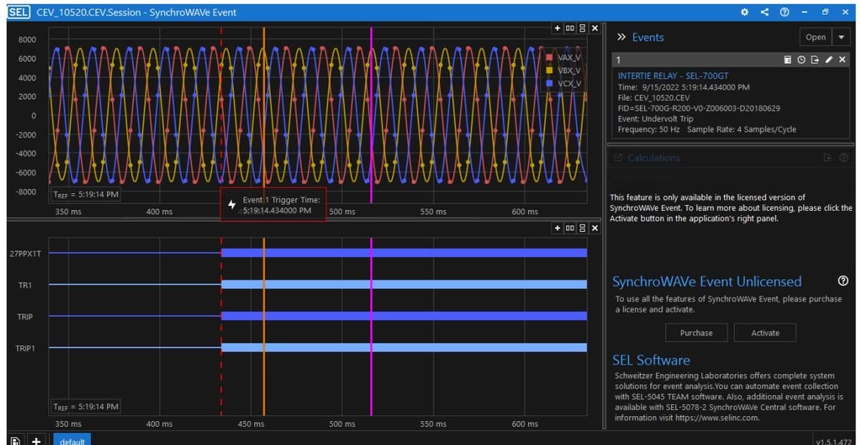
Figure 5. 21a: SynchroWAVE Event test results for Under-voltage stage 1
