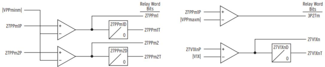
Figure 5. 14: Under voltage Element Logic (SEL-700G Instruction manual, 2015)
