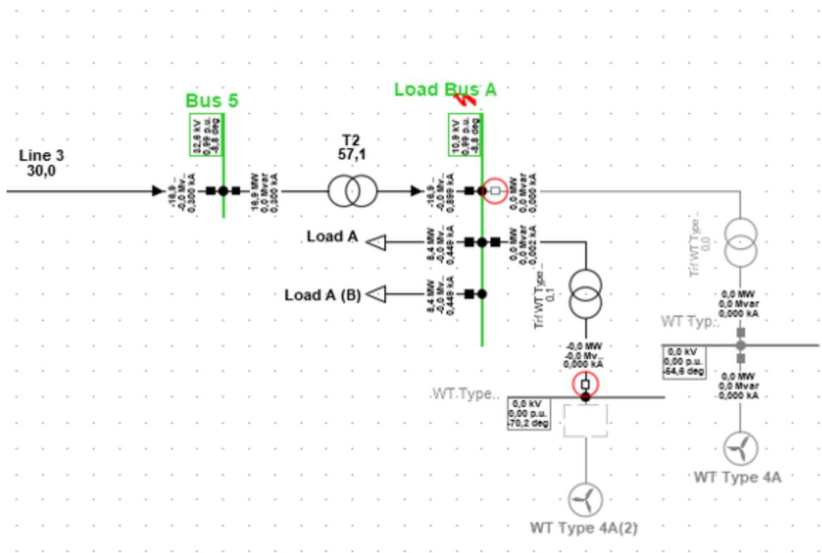
Figure 4. 12a: Phase A to Ground fault initiated on Load Bus A
