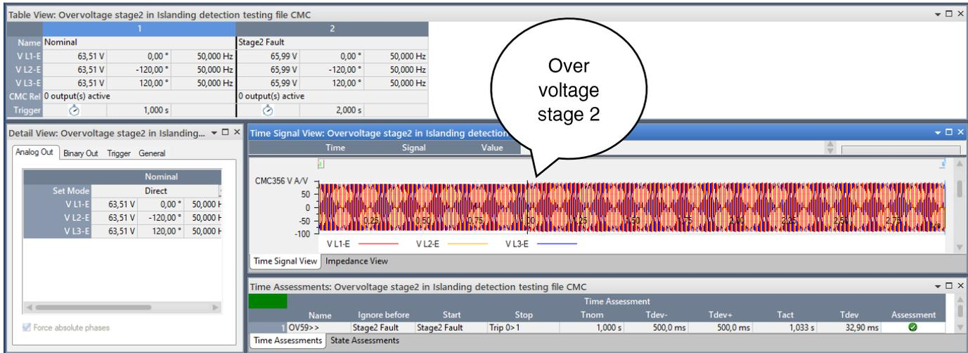
Figure 5. 19b: Test injection configuration for Over-voltage stage 2
