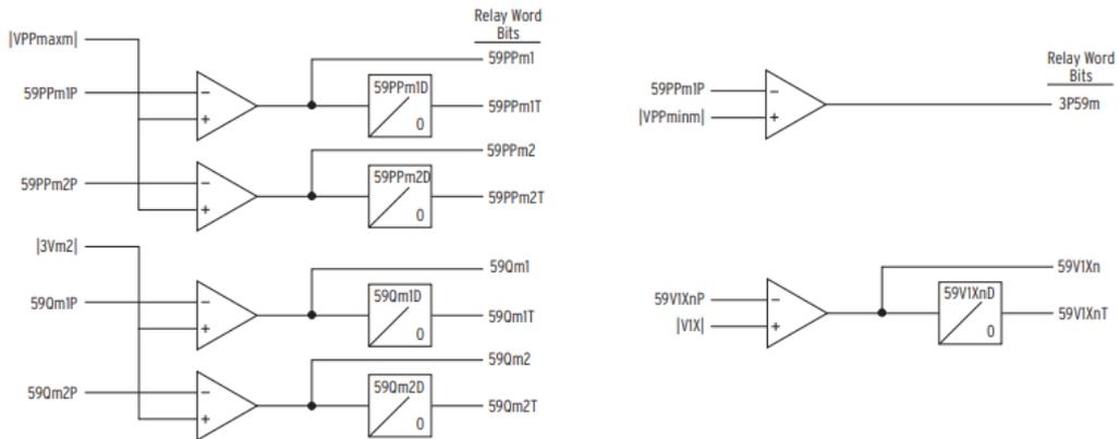
Figure 5. 15: Over voltage Element Logic (SEL-700G Instruction manual, 2015)
