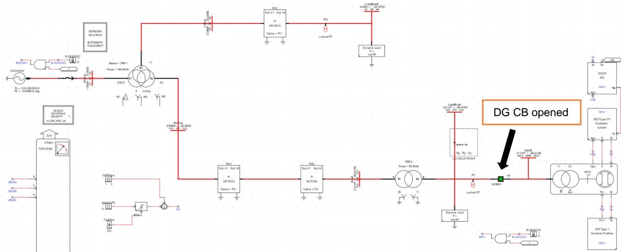
**Figure 6. 12: Grid-connected islanded mode**
