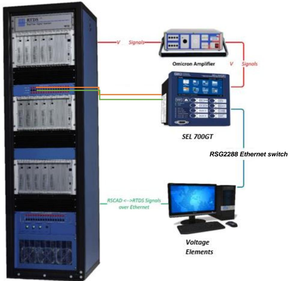
**Figure 6. 16: Hardware-in-the-Loop structure**
