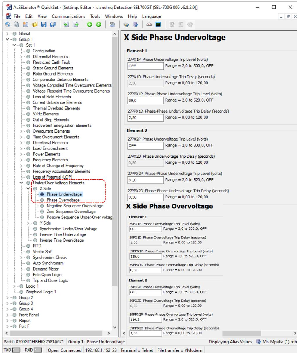
Figure 6. 21: Voltage Elements on the X Side of the SEL 700GT
