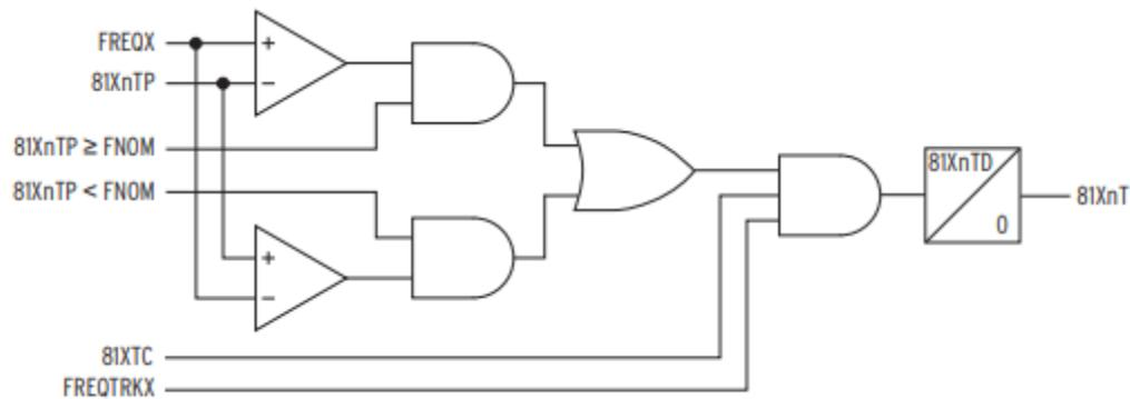
**Figure 5. 13: X-Side Over- and Underfrequency Element Logic (SEL-700G Instruction manual, 2015)**
