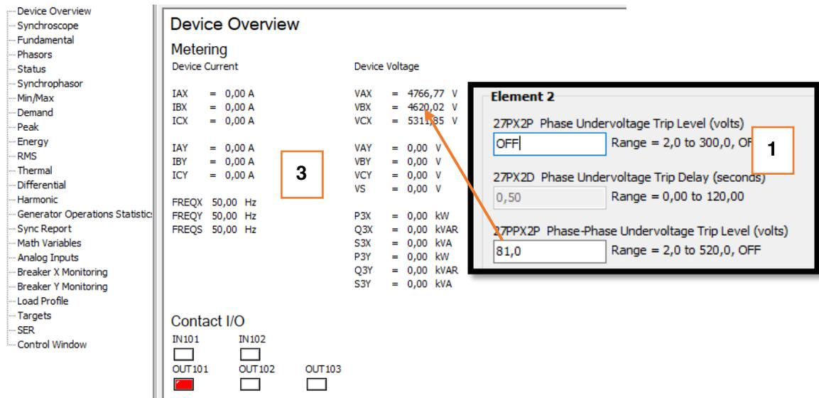
**Figure 6. 31c: Under voltage findings for stage 2 are displayed on the HMI display by monitoring relaying output port OUT101**
