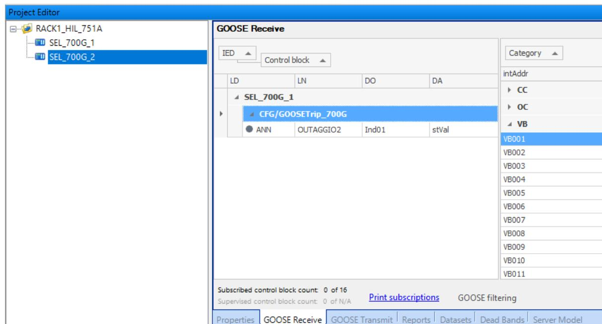
Figure 6. 42: GOOSE configuration on AcSELERator Architect
