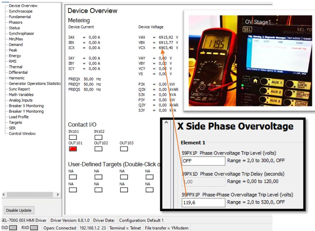
Figure 6. 34c: Over voltage findings for stage 1 are displayed on the HMI display by monitoring relaying output port OUT101
