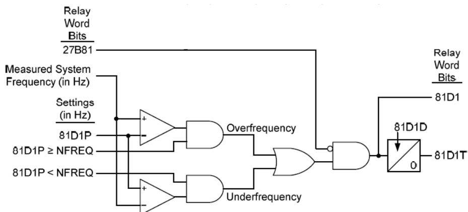
Figure 3. 8: Frequency logic (SEL-700G Instruction manual, 2015)
