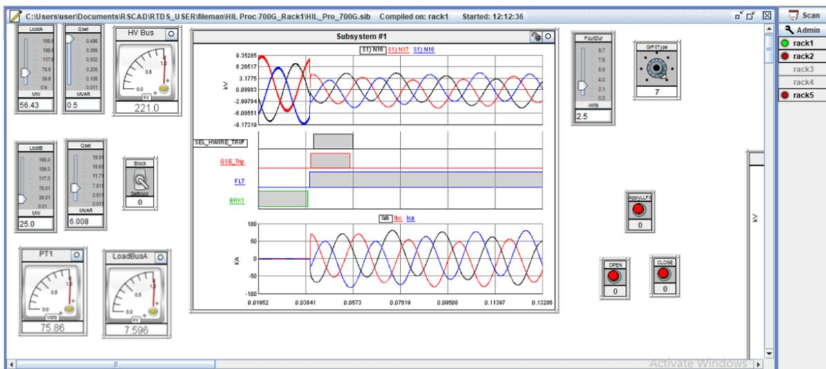
**Figure 6. 46: GOOSE response when three phase short circuit fault applied on feeder A**
