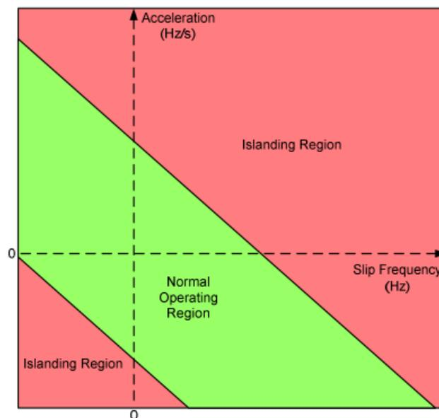
Figure 3. 6: Islanding detection characteristic using wide area measurements (Mulhausen et al., 2010)
