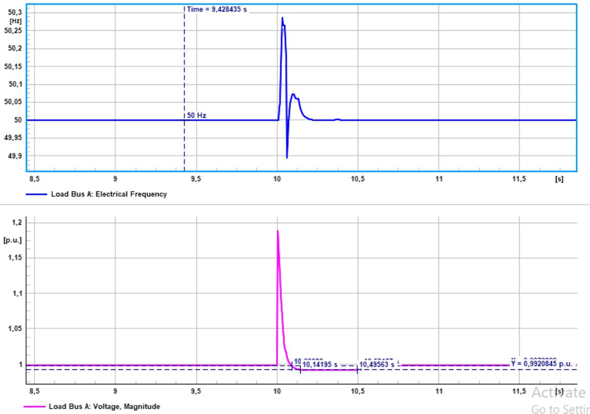
Figure 4. 6: System response when the grid-connected system isolates and wind turbines supplying microgrid connected system.
