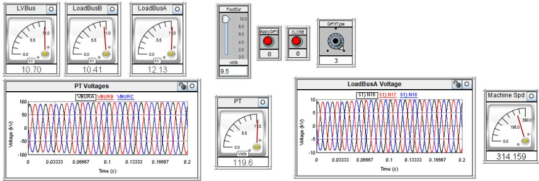
Figure 6.32a: Runtime Over Voltage results for stage 1
