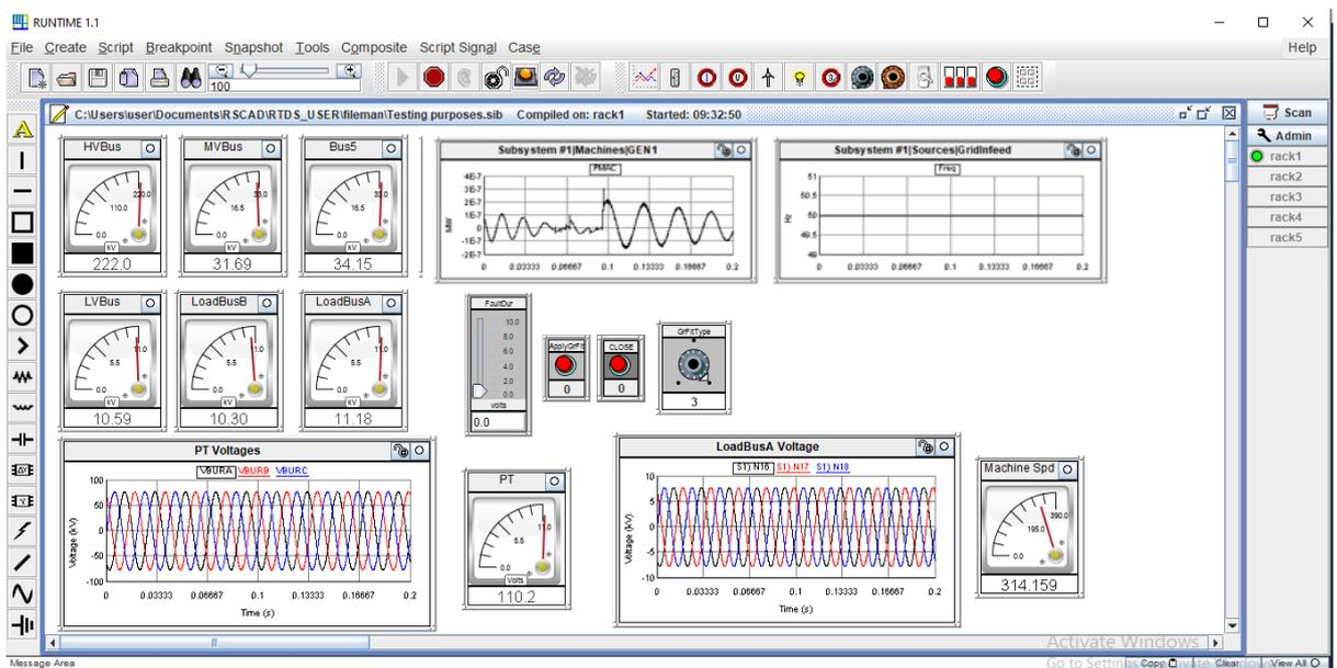
Figure 6. 25: Runtime displaying Node voltages and logic controllers
