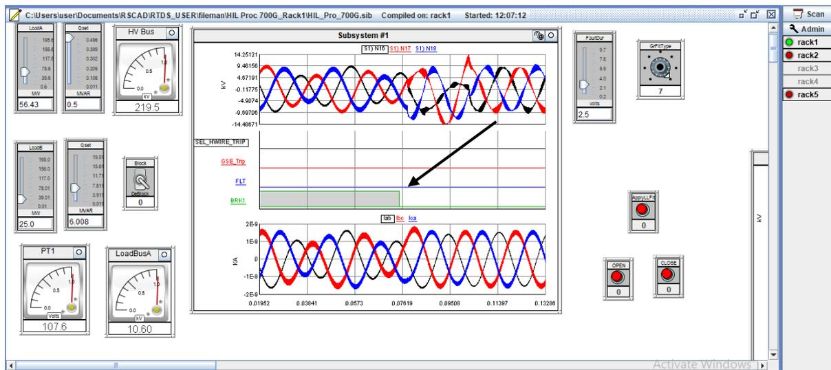
Figure 6. 44: Circuit breaker BRK1 shows open state
