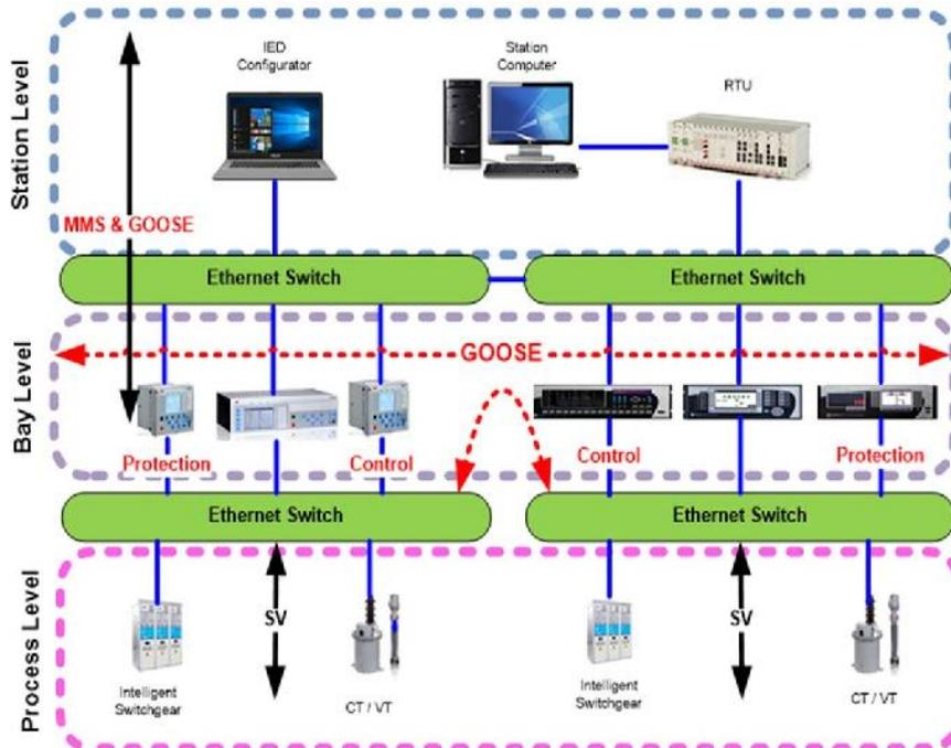
Figure 2. 7: Communication network architecture (Kulkarni et al., 2015)
