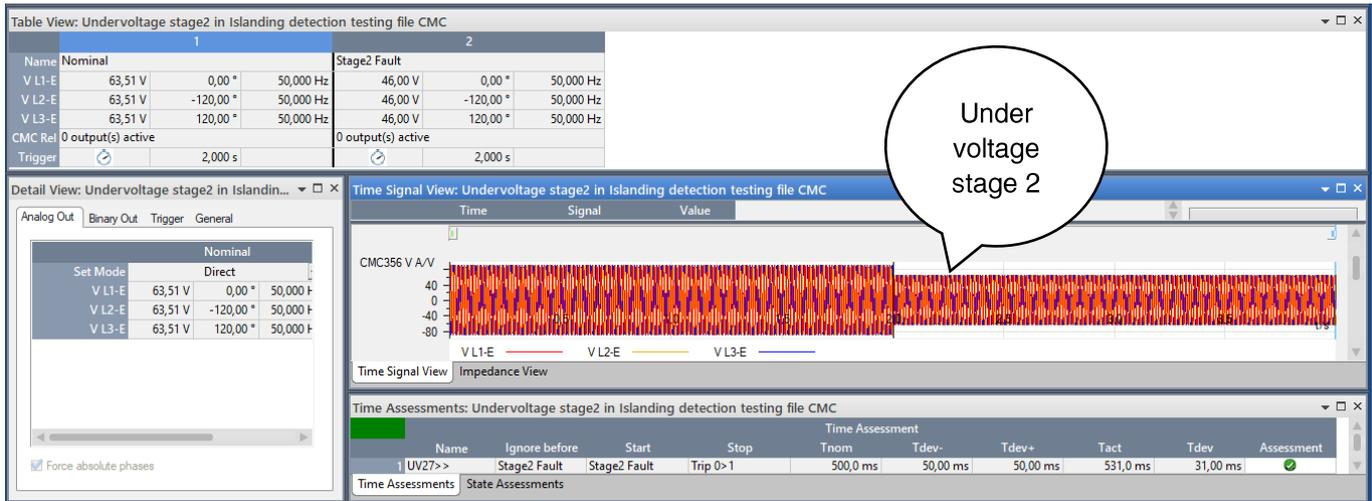
Figure 5. 17b: Test injection configuration for Under-voltage stage 2
