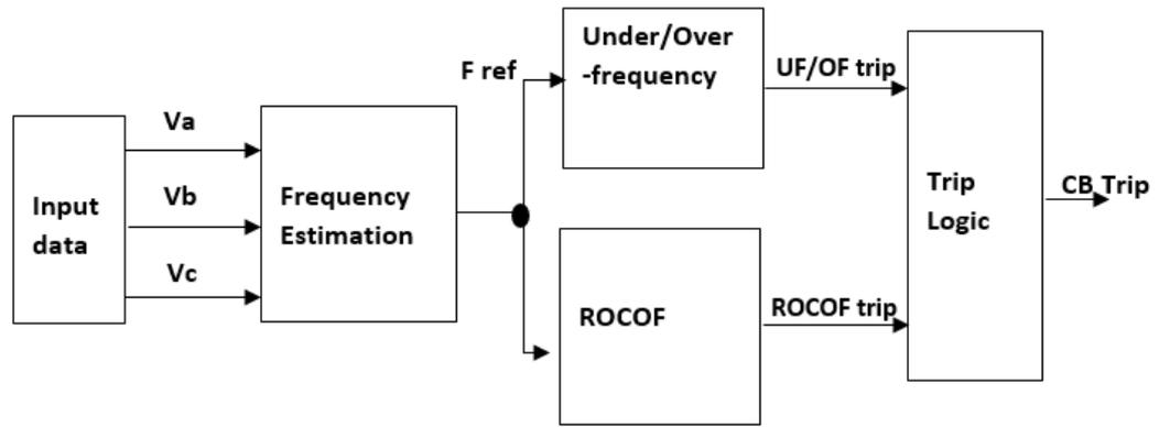
Figure 4. 8: Structure diagram for the protection functions (OF, UF and ROCOF)(Elvis et al., 2020)
