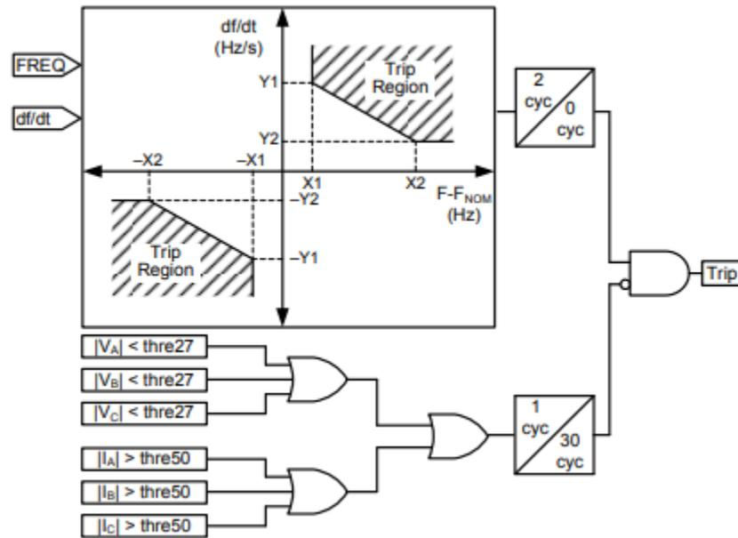
Figure 3. 5: IDS using local measurements (Mulhausen et al., 2010)
