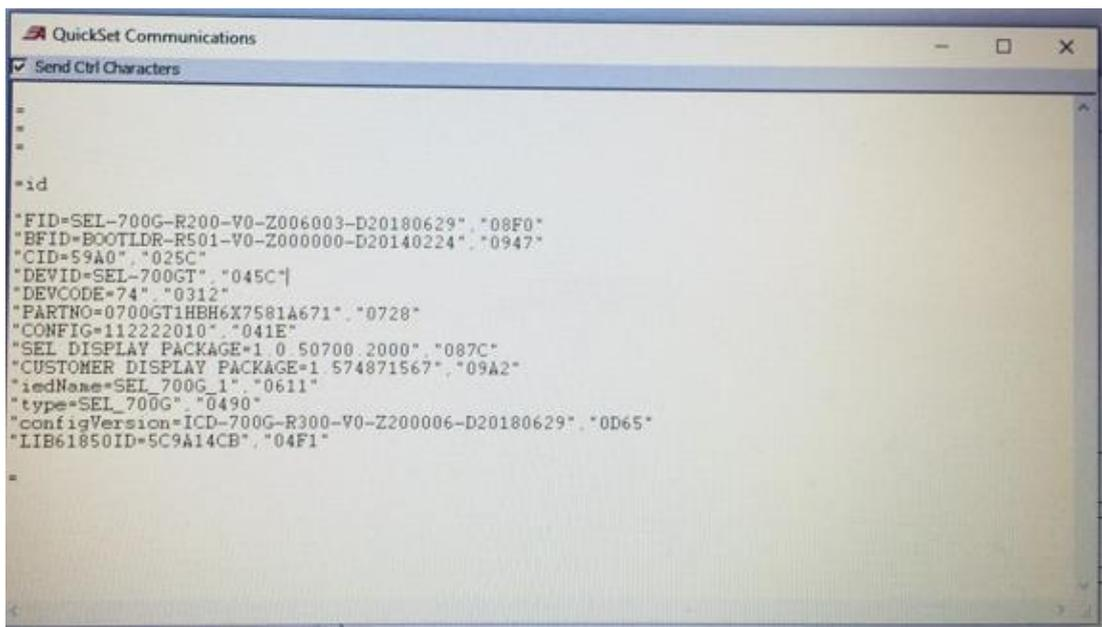
Figure 5. 6: SEL700GT generator protection relay response communication
