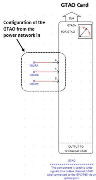
**Figure 6. 3: GTA0 card under draft module**
