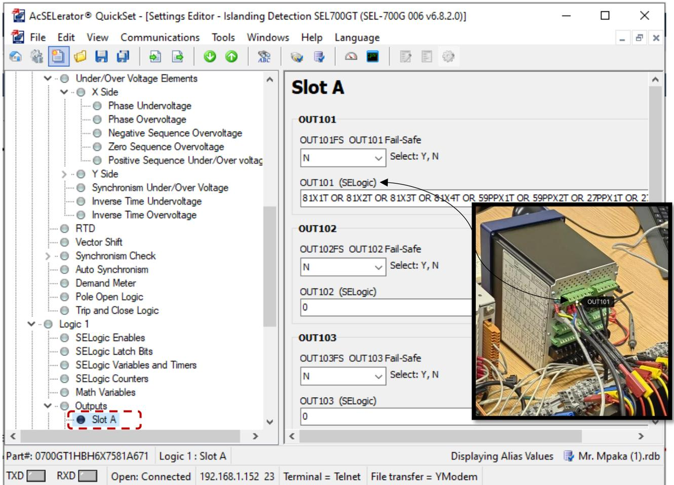
Figure 6. 22: Logic 1 Slot A Voltage elements and Frequency elements
