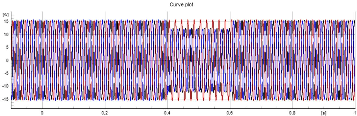
**Figure 4. 13b: Voltage waveform during Under-Voltage**
