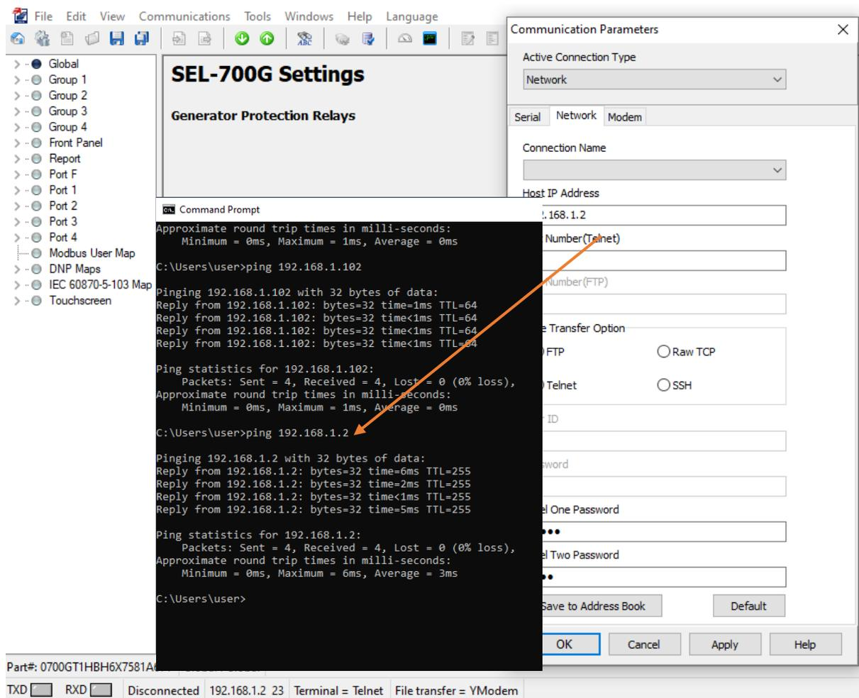
Figure 6. 6: RTDS and PC ping command results for SEL700GT and RTDS racks.
