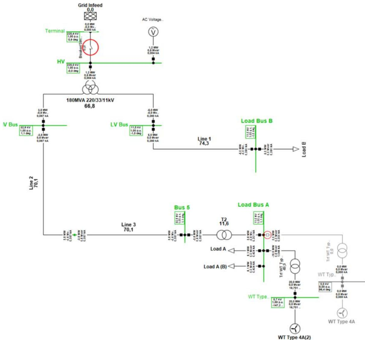
Figure 4. 5: Microgrid-connected islanded operations
