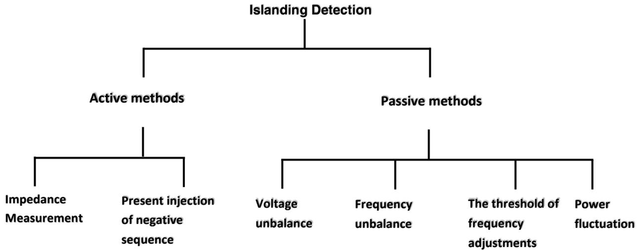
**Figure 2. 6: Block Diagram for islanding detection methods (Active and passive)**
