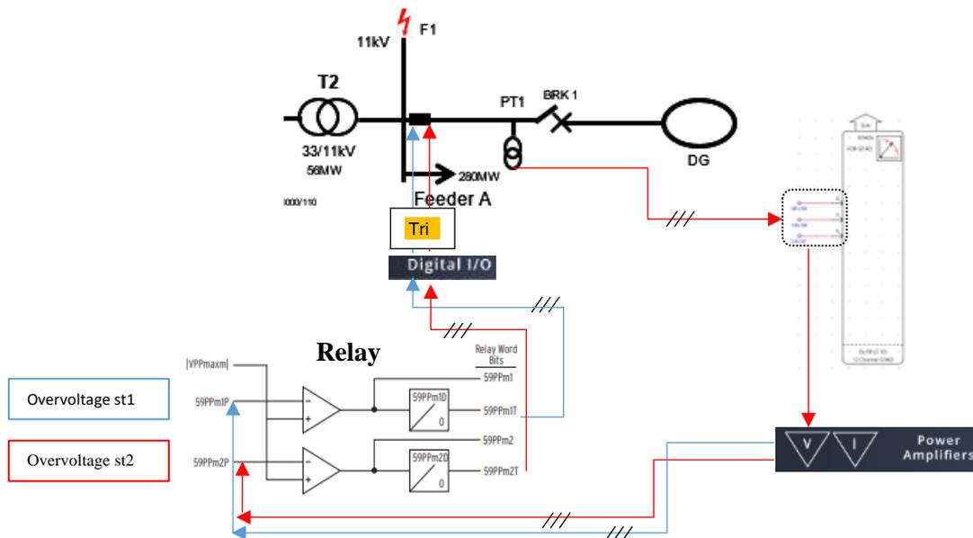
Figure 6. 24: OV protection functions
