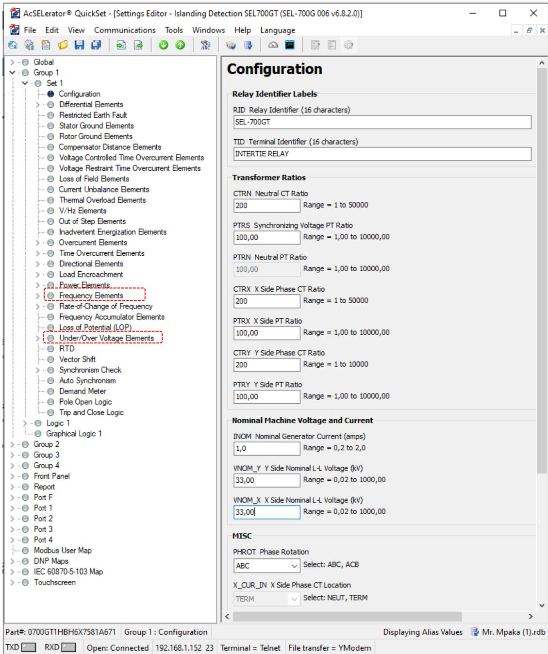
Figure 6. 20: Configure the SEL700GT's frequency and under/overvoltage elements.
