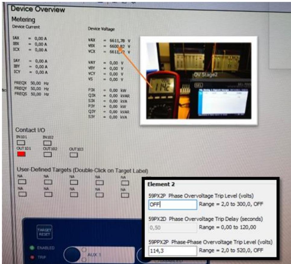
Figure 6. 37c: Relay settings for over voltage stage2
