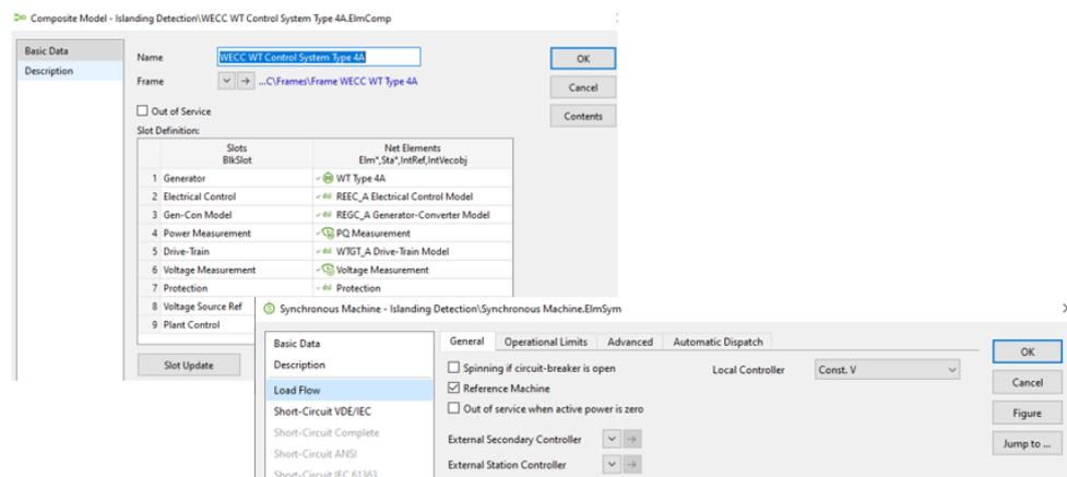
Figure 4. 14: Synchronous Machine as reference instead of External grid
