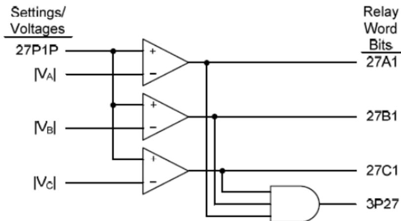
Figure 3. 7: Under-voltage logic (SEL-700G Instruction manual, 2015)
