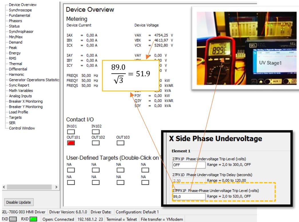
Figure 6. 28c: UV findings for stage 1 are displayed on the HMI display by monitoring relaying output port OUT101
