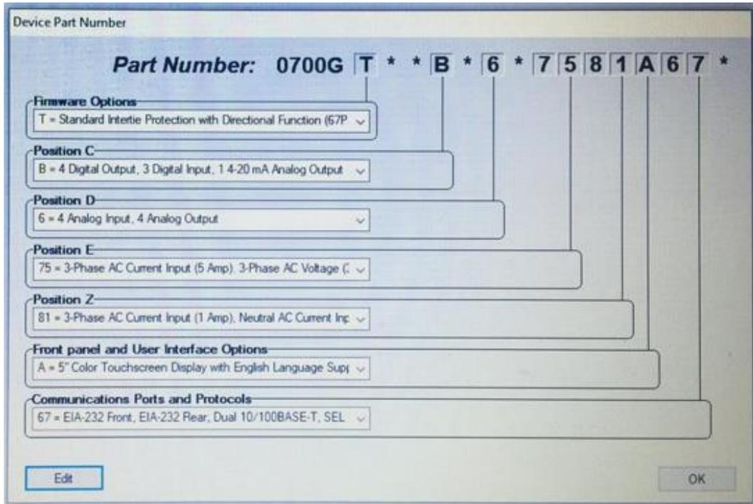
Figure 5. 5: SEL700GT generator protection relay Part Number
