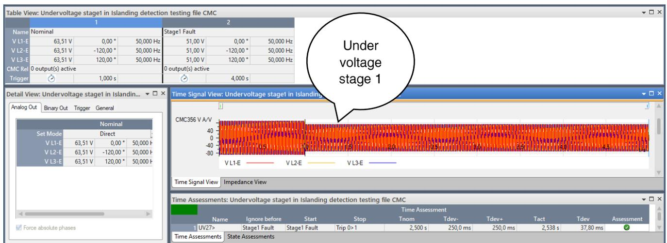
Figure 5. 16a: Test injection configuration for Under-voltage stage 1
