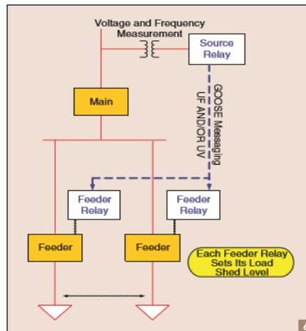
**Figure 2. 8: A load scheme with GOOSE messaging (Sevov et al., 2013)**
