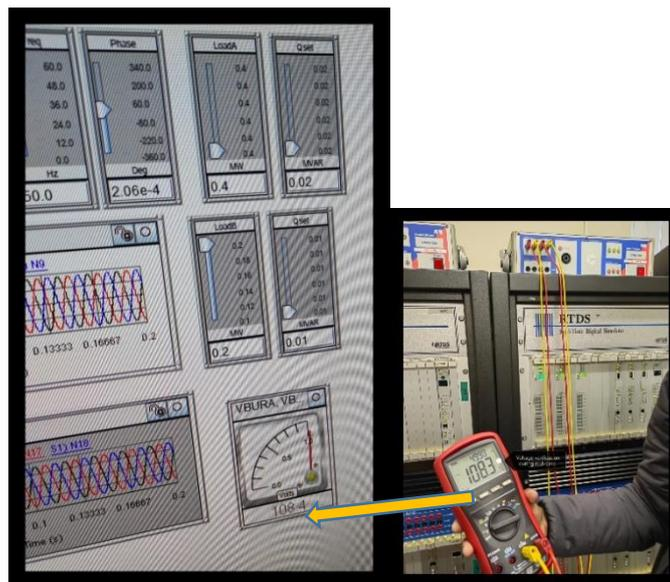
Figure 6. 18: Voltage verification on the PT connected next to the LoadbusA
