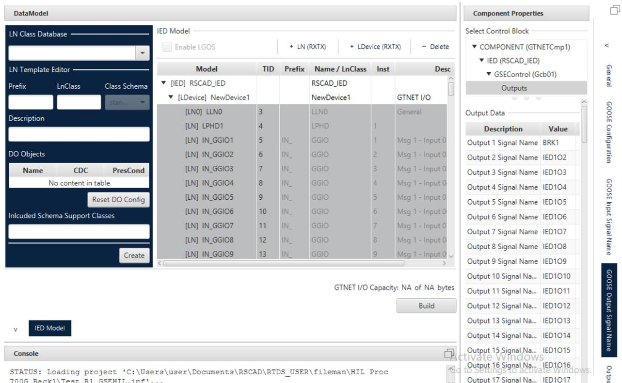
Figure 6. 41: IEC 61850 GOOSE messaging from the RTDS simulator using the new ICT tool in RSCAD-FX
