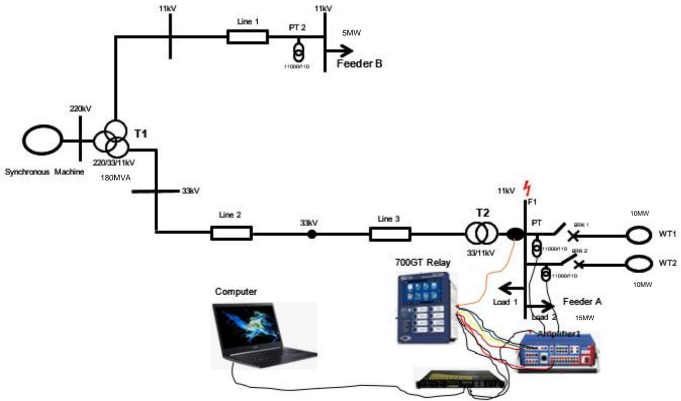
Figure 5. 2: lab-scale testing of the islanded protection scheme set up
