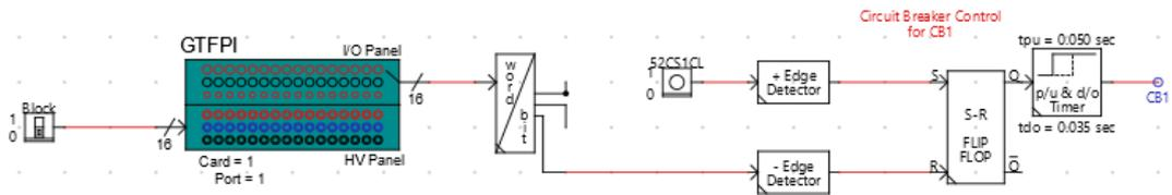
Figure 6. 9: GTFPI control logic technique for circuit breakers
