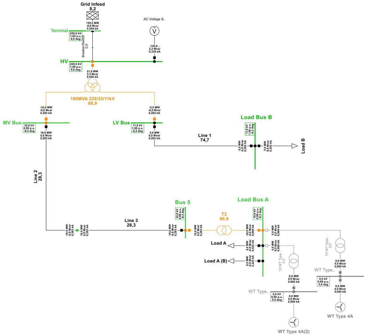
Figure 4. 9: Distribution network at normal state
