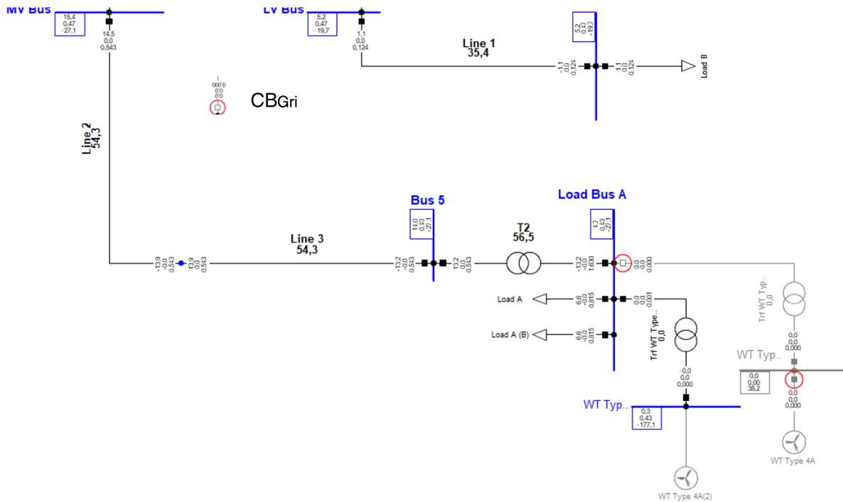
Figure 4. 21: CBGrid opened to create Over-frequency condition
