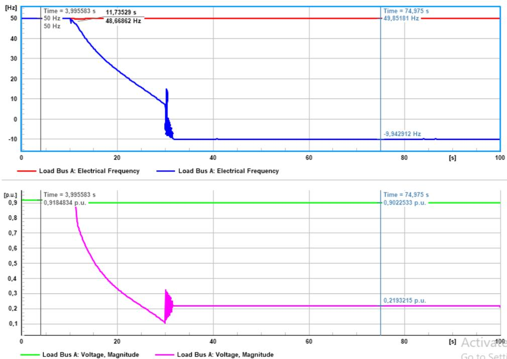
Figure 4. 19: System collapsed as external grid used as reference
