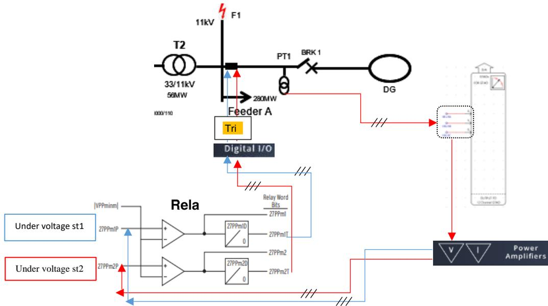
Figure 6. 23: UV protection functions
