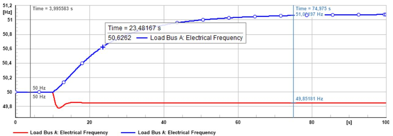
Figure 4. 22: Over frequency condition when the CBGrid tripped
