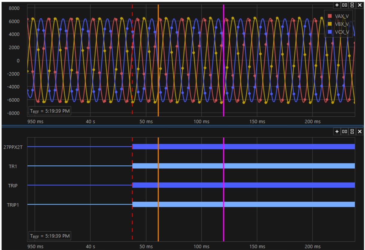
**Figure 5.22b: SynchroWAVE Event test results for Under-voltage stage 2**
