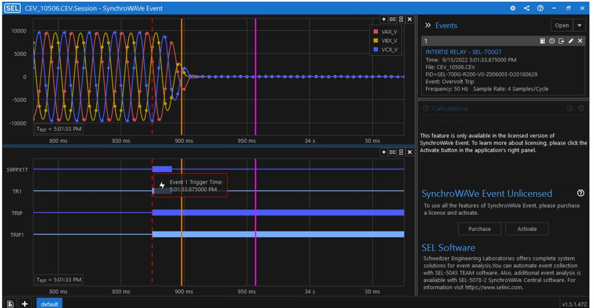
Figure 5. 23a: SynchroWAVE Event test results for Overvoltage stage 1
