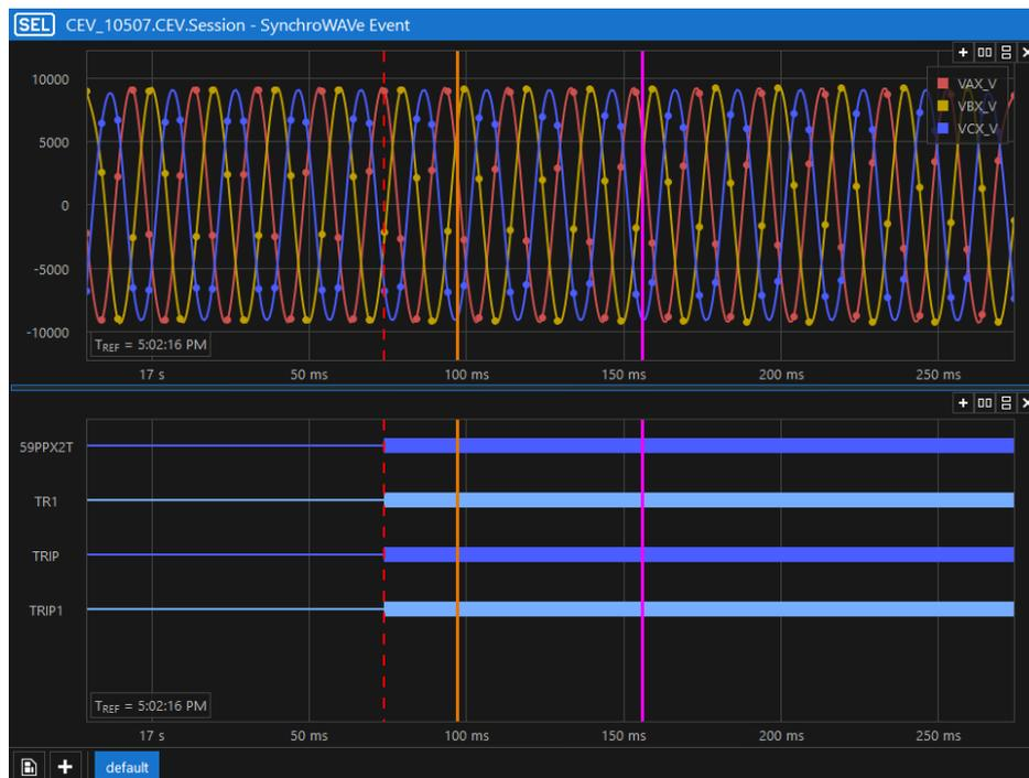
Figure 5. 24b: SynchroWAVE Event test results for Overvoltage stage 2
