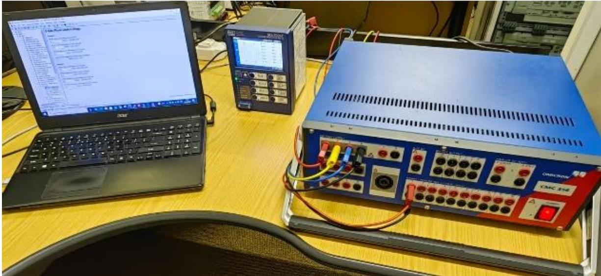
Figure 5. 3: Physical layout lab-scale testing of islanding protection scheme set up
