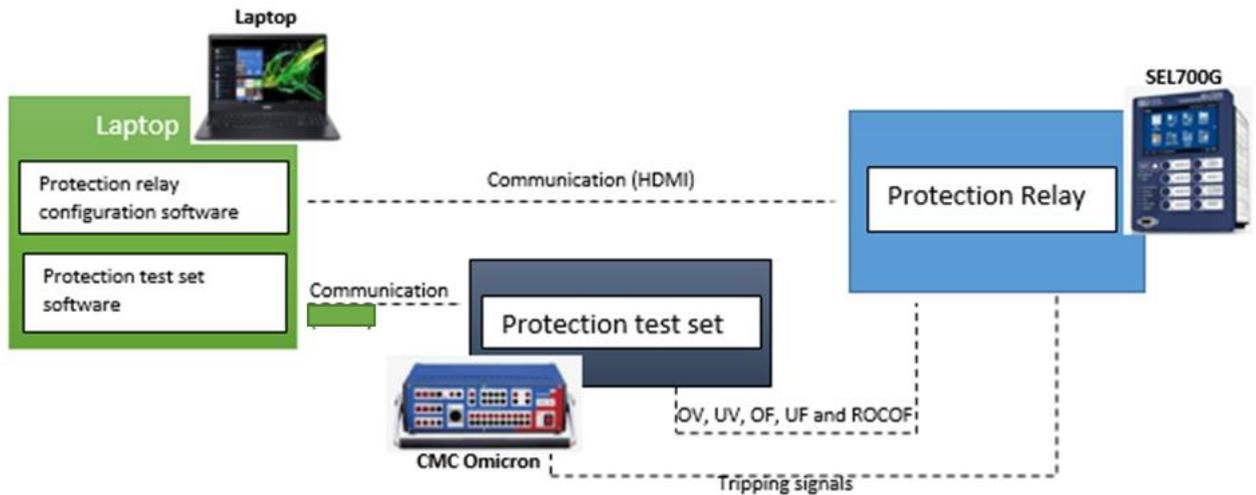
**Figure 5. 4: Static type testing hardware environment**
