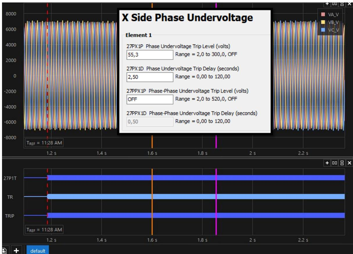
Figure 6. 47: Under voltage results and relay operating time
