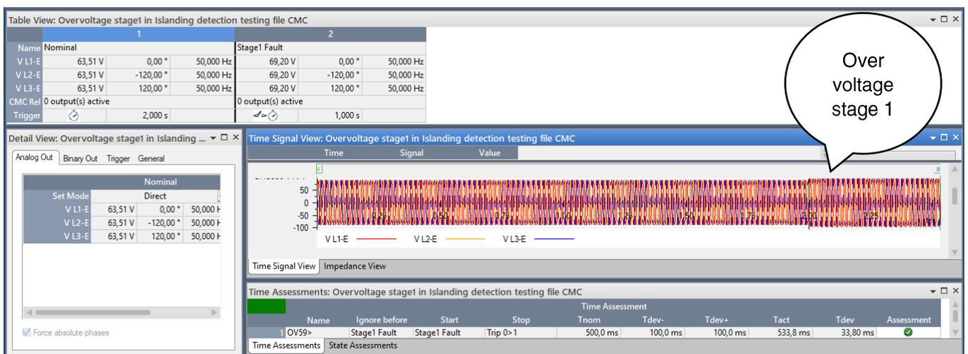
Figure 5. 18a: Test injection configuration for Over-voltage stage 1
