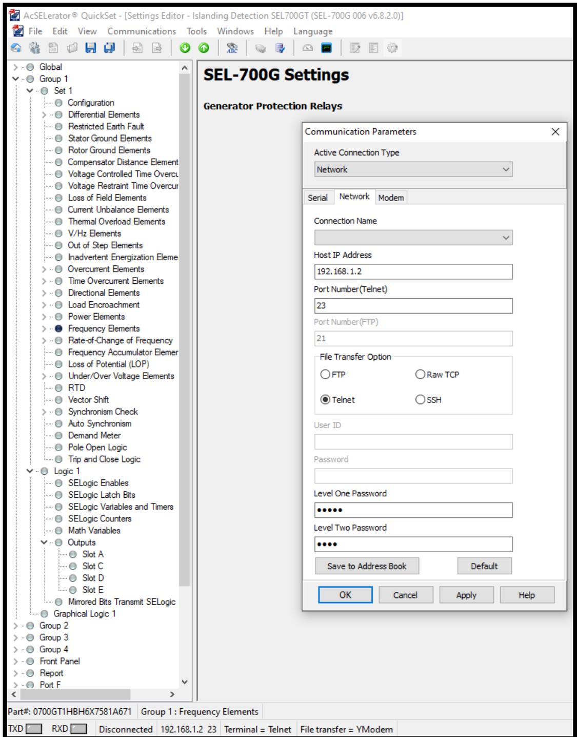
**Figure 5. 7: SEL700GT communication parameter settings**
