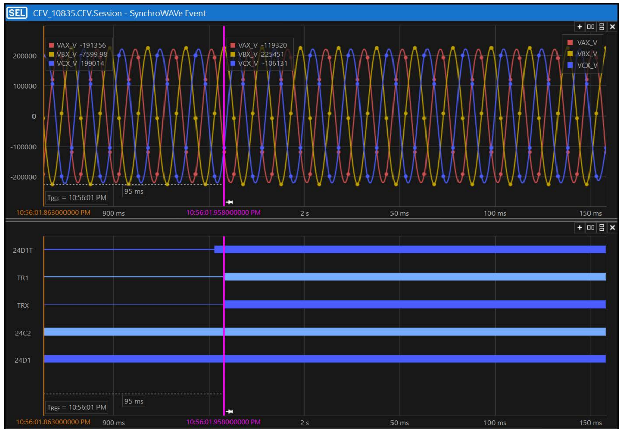
Figure 5.22: Phase to phase voltages and trip signals of the SEL 700G at V/Hz level of 120%
