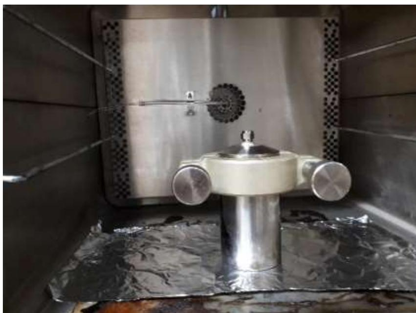
**Figure 3.2: 200 mL pressure vessel inside oven**
