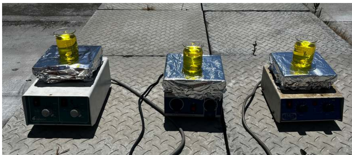
Figure 3.2: The experimental setup for the photocatalytic evaluation of solar illumination
