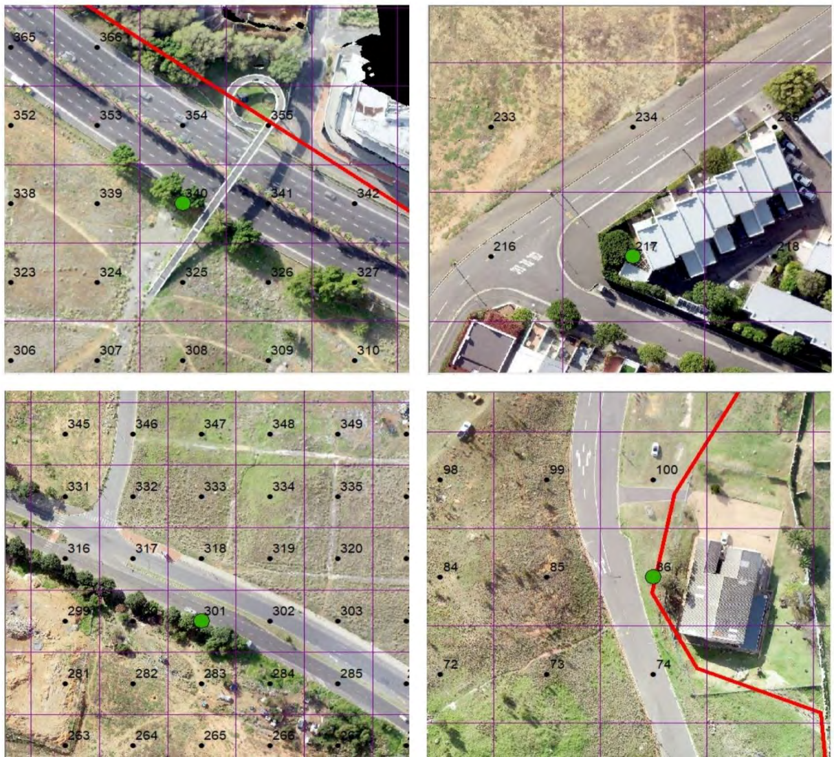
FIGURE 4.20: EXAMPLE OF OUTLIERS FROM THE 30X30M GRID FOR RELATIVE ACCURACY
