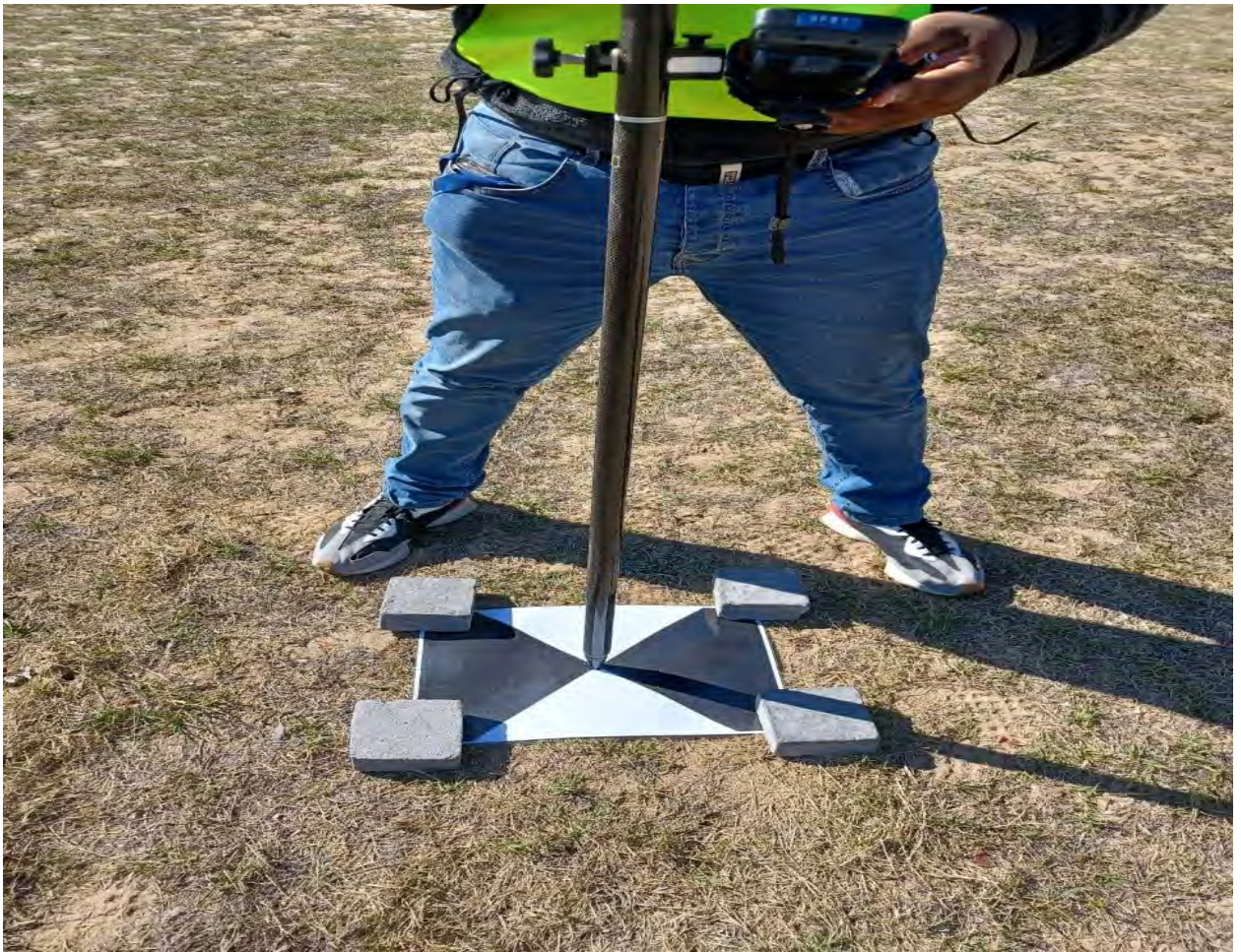
FIGURE 3.11: LOCATION OF GROUND CONTROL POINTS USING GPS
