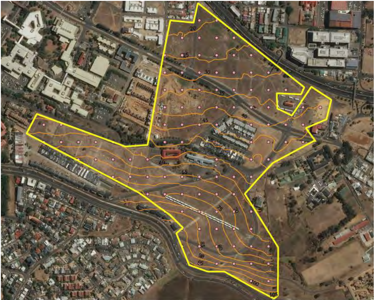
FIGURE 3.6: CHECK POINTS DISTRIBUTION, DIGITISED CONTOUR LINES
