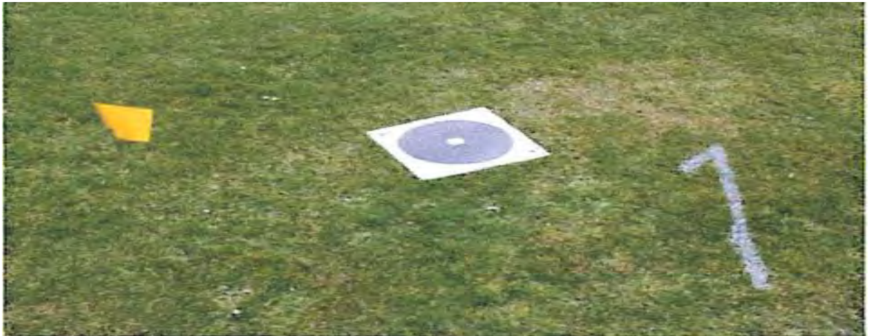
FIGURE 2.7: GROUND CONTROL AND CHECK POINT TARGET
