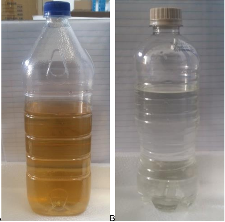
Photograph3.2: Initial groundwater before treatment in A and after treatment B
