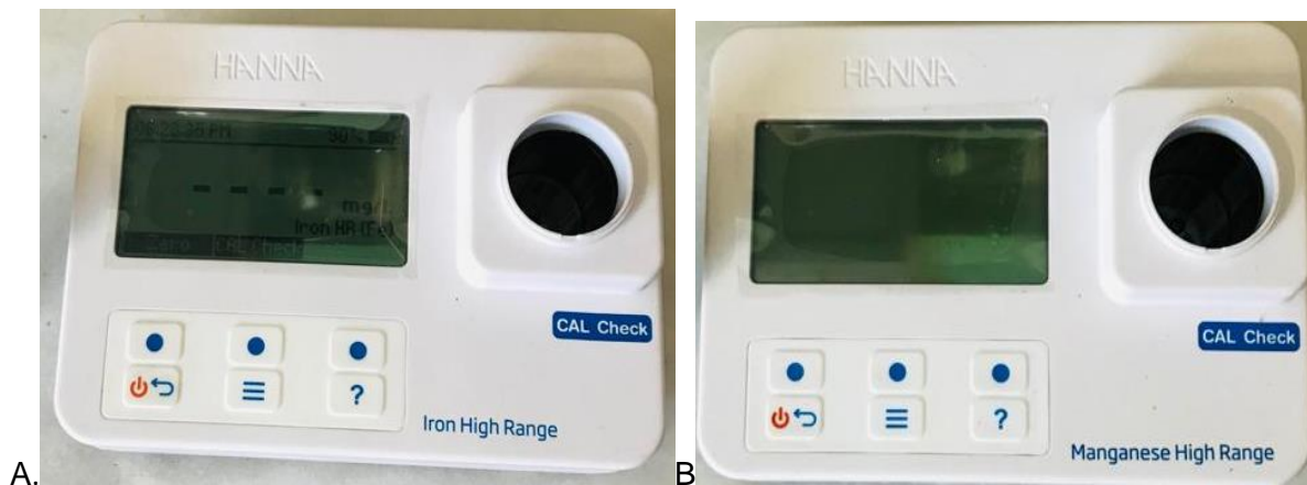
Photograph 3.3A: HI97721C Iron testing and Photograph 3-3B HI97709C Manganese High range testing meter,
