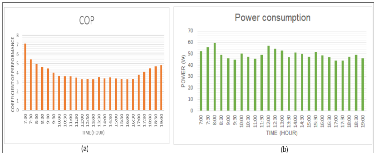
Figure 5. 11: (a) the coefficient of performance of VC heat pump system; (b) the energy consumption of the DC compressor
