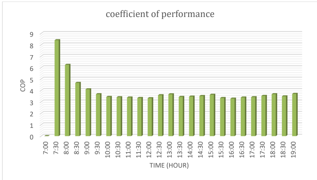
Figure 5. 21: The COP of vapour compression heat pump system on 14 July
