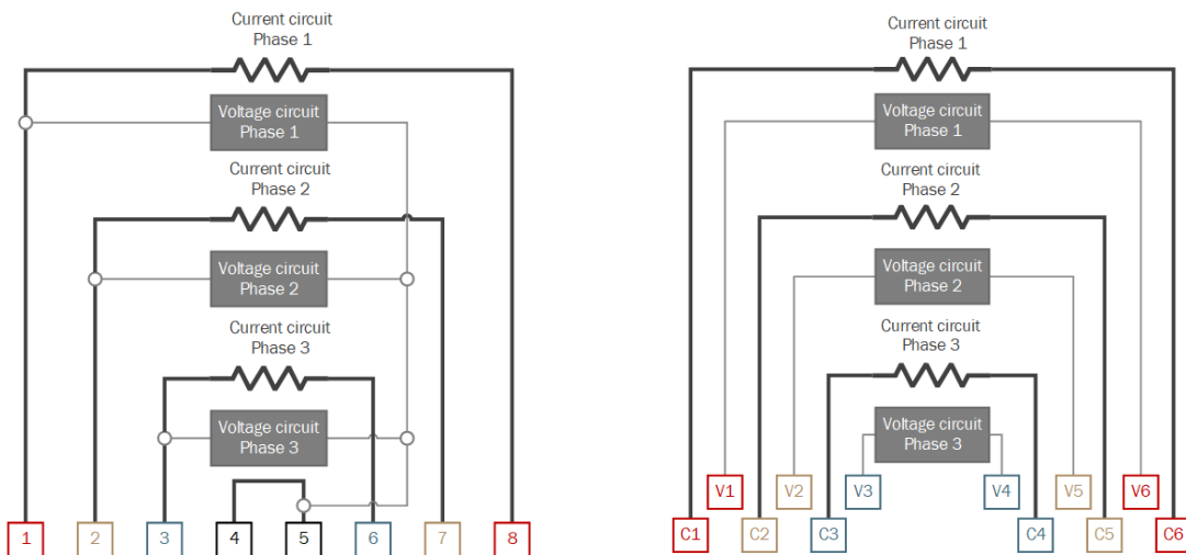
Figure A.2: Connection to the grid, left-to-right: Direct meter circuit, and indirect meter circuit, current transformers, voltage transformers (based on Toledo (2013))
