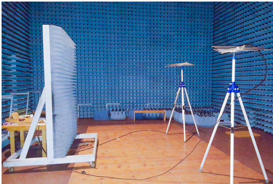
Figure 2.9: Houwteq anechoic chamber. The walls, roof and floor (under the wood shown) are lined with radar absorbing material.
